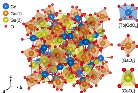
Fig. 3 Crystalline structure of body-centered cubic Gd<sub>3</sub>Ga<sub>5</sub>O<sub>12</sub>:Tb (sp. gr.  $Ia\bar{3}d - O_h^{10}$ ) after the description reported in the literature:<sup>33,34</sup> (left) a fragment of the structure within a single unit-cell (black lines); (right) the coordination polyhedra [Tb|GdO<sub>6</sub>], [GaO<sub>6</sub>] and [GaO<sub>4</sub>].
