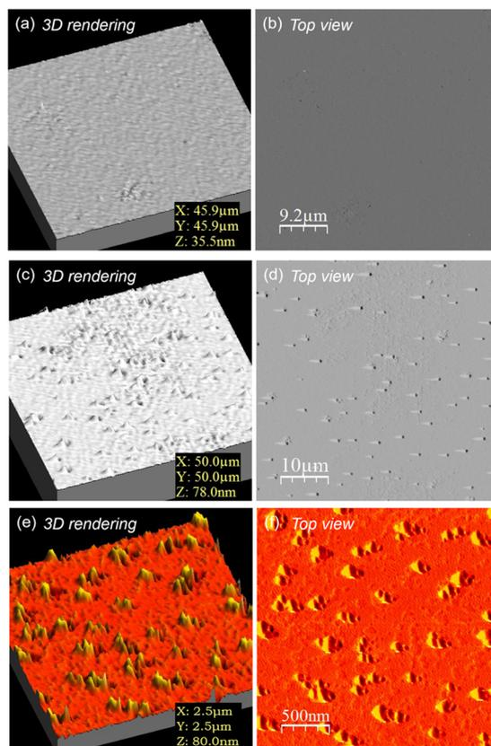
Fig. 7 Atomic force microscopy images of the as-grown faces of a GGG:Tb layer (epitaxy no. 8): (a and b) the upper face over a  $50 \times 50 \mu\text{m}^2$  area: (a) 3D rendering, (b) top view; (c and d) the down face over a  $50 \times 50 \mu\text{m}^2$  area: (c) 3D rendering, (d) top view; (e and f) the down face over a  $2.5 \times 2.5 \mu\text{m}^2$  area: (e) 3D rendering, (f) top view.
