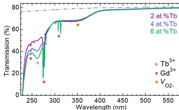
Fig. 9 Transmission spectra of GGG:Tb epitaxies no. 3, 5 and 7 with 2 at%, 4 at%, and 6 at%  $\text{Tb}^{3+}$  in the flux, respectively, in the UV-visible spectral range. Symbols – contributions of  $\text{Gd}^{3+}$  and  $\text{Tb}^{3+}$  ions, and compensation of the oxygen vacancies  $\text{V}_{\text{O}^{2-}}$ , dashed grey line – theoretical limit  $T_0$  set by Fresnel losses after Wood and Nassau.<sup>42</sup>
