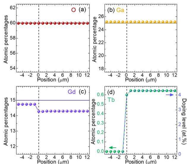
Fig. 5 Percentages of atoms for the different constituents across the GGG:Tb epitaxy no. 4 with 4 at%  $\text{Tb}^{3+}$  in the flux: (a) O; (b) Ga; (c) Gd; (d) Tb. Positive positions correspond to the  $12.7$  μm-thick  $\text{Tb}^{3+}$ -doped layer, and negative ones – to the GGG substrate. Dashed vertical lines – the layer/substrate interface. Solid horizontal lines – the stoichiometric composition for undoped GGG.
