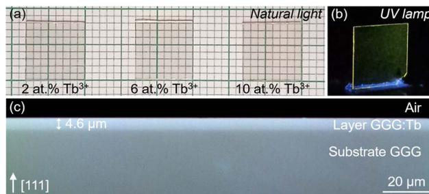
Fig. 1 As grown GGG:Tb/GGG epitaxies: (a) photographs under natural light (epitaxies no. 3, 7, and 10, with 2 at%, 6 at%, and 10 at% Tb<sup>3+</sup> in the flux, respectively); (b) a photograph under UV illumination,  $\lambda_{\text{exc}} = 313$  nm (epitaxy no. 7); (c) a confocal laser microscopy image of an end-facet (epitaxy no. 7) using a  $\times 50$  objective.
