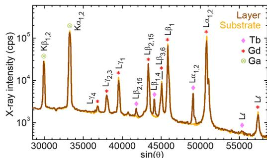
Fig. 6 Comparison of the WDS spectra of a GGG substrate and a Tb<sup>3+</sup>-doped layer (epitaxy no. 4 with 4 at% Tb<sup>3+</sup> in the flux). Symbols – contributions of Gd, Tb and Ga assigned using experimental data reported in the literature.<sup>37,38</sup>
