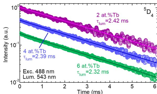
Fig. 11 Photoluminescence decay curves from the  $^5\text{D}_4$  state of  $\text{Tb}^{3+}$  ions in GGG:Tb layers with various doping levels (epitaxies no. 3, 5 and 6, with 2 at%, 4 at%, and 6 at%  $\text{Tb}^{3+}$  in the flux, respectively).  $\lambda_{\text{exc}} = 488$  nm,  $\lambda_{\text{lum}} = 543$  nm. Circles – experimental data, lines – linear fit,  $\tau_{\text{lum}}$  – luminescence lifetime of the  $^5\text{D}_4$  emitting state of  $\text{Tb}^{3+}$  ions.
