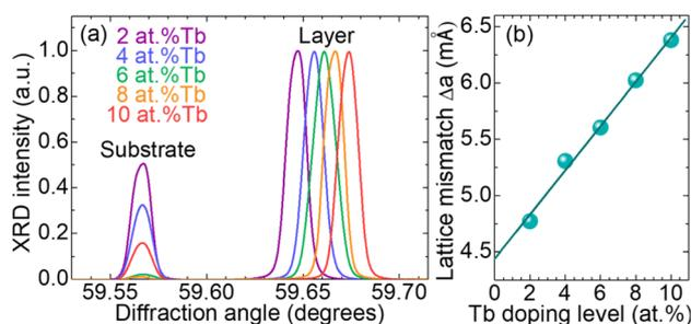
Fig. 4 Influence of the Tb doping level on the lattice mismatch between the GGG substrates and the doped epitaxial layers: (a) X-ray diffraction ( $\omega$ ,  $2\theta$ ) scans at the (888) reflection; (b) linear relation between the lattice mismatch and the Tb content.
