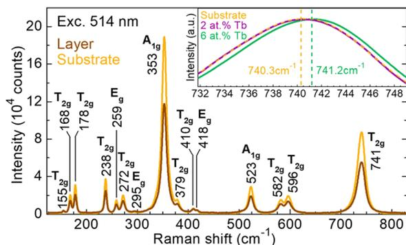
Fig. 8  $\mu$ -Raman spectra of a GGG substrate and layer doped with 2 at%  $\text{Tb}^{3+}$  (epitaxy no. 3). The inset shows a close look at the Raman peak at  $741\text{ cm}^{-1}$  for a GGG substrate and layers doped with 2 at% and 6 at%  $\text{Tb}^{3+}$  (epitaxies no. 3 and 6, respectively).  $\lambda_{\text{exc}} = 514\text{ nm}$ . Numbers – Raman frequencies in  $\text{cm}^{-1}$ .
