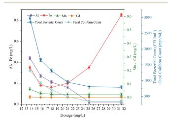
Fig. 14 Effect of coagulant dosage on supernatant Al, Fe, Mn, Cd, total bacterial counts and fecal coliform counts.
