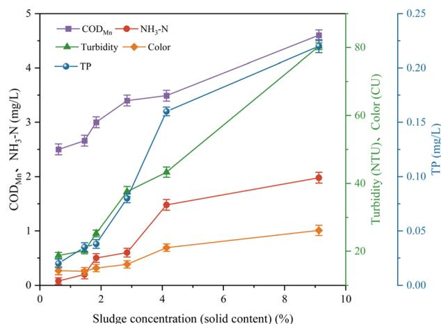
Fig. 11 Effect of discharge water concentration on COD<sub>Mn</sub>, NH<sub>3</sub>-N, TP, turbidity and color of supernatant liquid.
