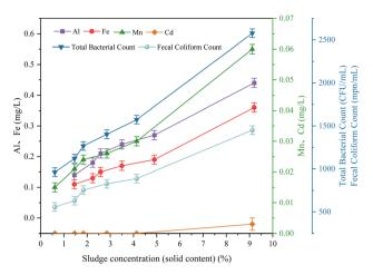
Fig. 12 Effect of discharge water concentration on supernatant Al, Fe, Mn, Cd, total bacteria and fecal coliform counts.
