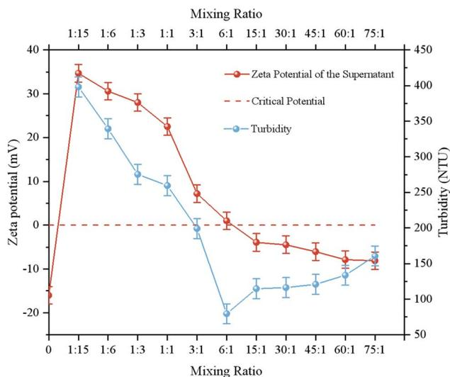
Fig. 15 Zeta potential of supernatant after adding different mixing ratios of coagulants.
