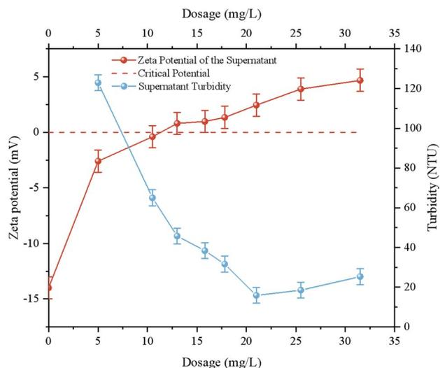
Fig. 16 Zeta potential of supernatant after treatment with different dosages of the coagulant.
