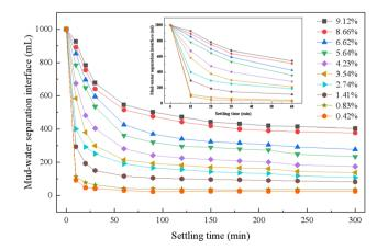
Fig. 1 Natural settling curves for different concentrations of drainage water.
