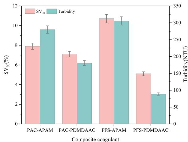
Fig. 4 Effect of different composite coagulant combinations on the coagulation effect.
