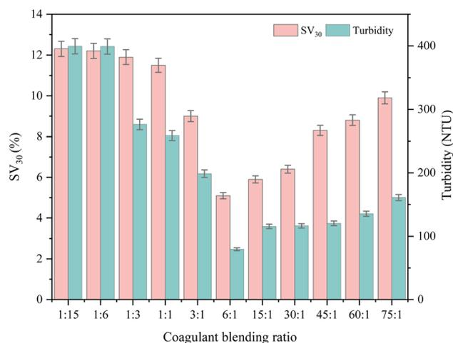
Fig. 5 Impact of different PFS–PDMDAAC composite coagulant ratios on coagulation performance.
