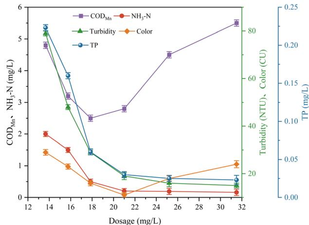
Fig. 13 Effect of coagulant dosage on COD<sub>Mn</sub>, NH<sub>3</sub>-N, TP, turbidity and color of supernatant solution.
