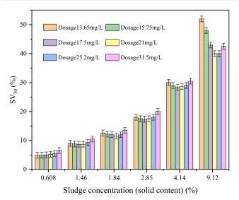
Fig. 10 Effect of discharge water concentration and dosage on sludge settleability after coagulation.
