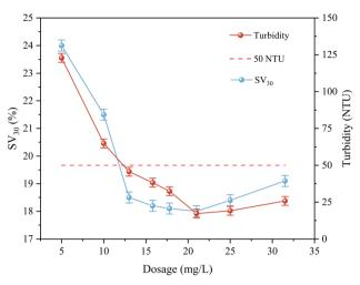
Fig. 6 Impact of different dosages of PFS-PDMDAAC composite coagulants on coagulation performance.
