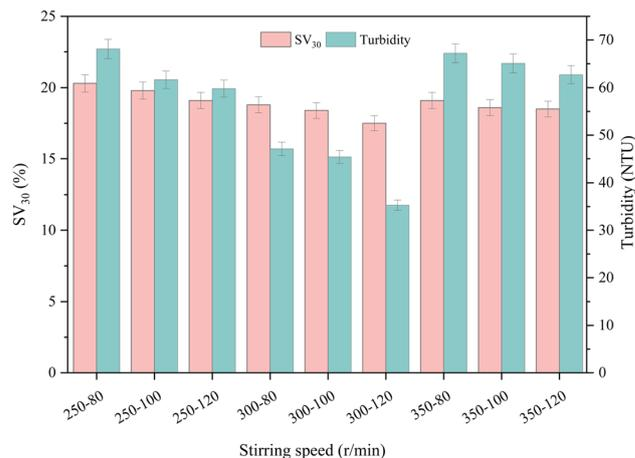
Fig. 7 Effect of different mixing speeds on the coagulation effect.
