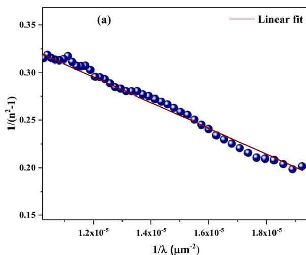
Fig. 12 Evolution of  $1/(n^2-1)$  versus: (a) the photon energy and (b)  $1/\lambda^2$ , relative to the  $(\text{C}_6\text{H}_9\text{N}_2)_3[\text{BiCl}_6]$  compound.
