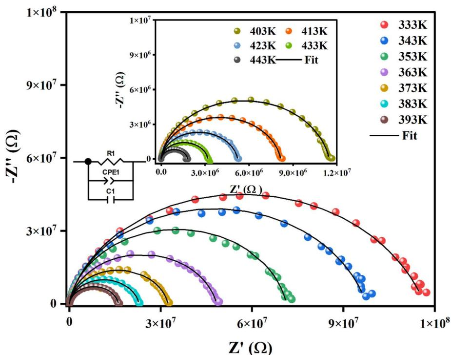
Fig. 14 Nyquist plots of  $(\text{C}_6\text{H}_9\text{N}_2)_3[\text{BiCl}_6]$  at different temperatures. The inset represents the equivalent circuit, and the calculated responses based on this circuit are given by the fitted lines.
