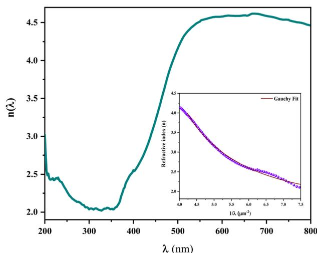
Fig. 11 Evolution of the refractive index  $n$  against wavelength  $\lambda$  (inset) fit of refractive index  $n$  using Cauchy's law.
