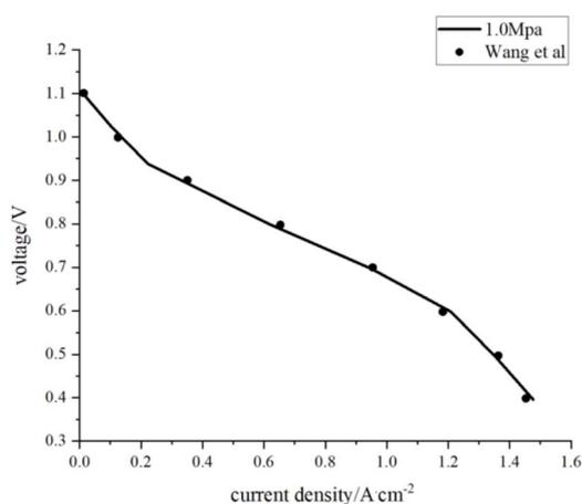
Fig. 4 Comparison between the simulated and experimental performance.
