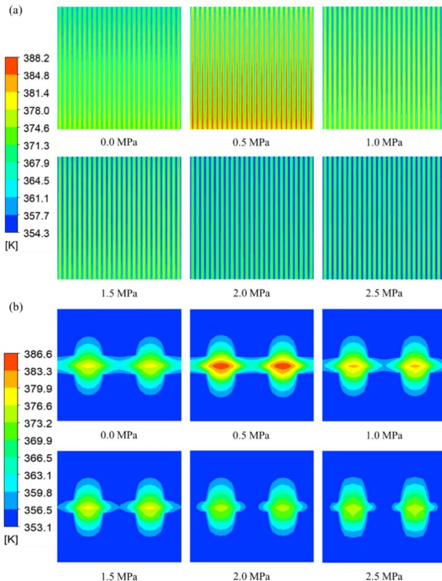
Fig. 6 Temperature distribution: (a) the interface of PEM and CL; (b) the xy cross-section of the fuel cell under the 12th and 13th channels.
