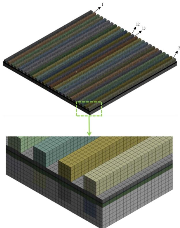
Fig. 2 Mesh diagram of the PEMFC under 0.5 MPa.
