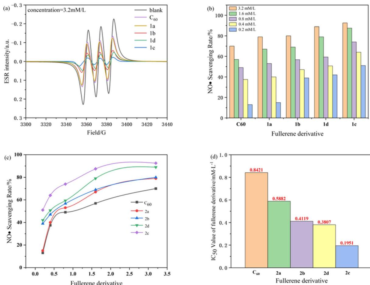
Fig. 8 (a) The ESR curves of compounds **2a–2d** and  $C_{60}$  at the  $3.2 \text{ mM L}^{-1}$  and blank sample; (b and c) NO· scavenging rates of compounds **2a–2d** and  $C_{60}$ ; (d)  $IC_{50}$  values of compounds **2a–2d** and  $C_{60}$  for the NO· scavenging rates.
