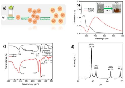
Fig. 1 (a) Schematic representation AgNPs formation using *Averrhoa bilimbi* fruit extract as reducing and stabilizing agents. (b) UV-visible spectra for *Averrhoa bilimbi* fruit extract and AgNPs and (d) X-ray Diffraction (XRD) pattern of AgNPs synthesized using AgNO<sub>3</sub> (1 mM, 40 mL) and *Averrhoa bilimbi* fruit extract (200 g  $L^{-1}$ , 1 mL) at 60 °C and pH = 10 for 30 min.
