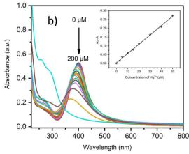
Fig. 5 (a) UV-vis absorption spectra of AgNPs solutions incubated with  $Hg^{2+}$  and other 14 metal ions at the same concentration (50  $\mu$ M) (b) UV-vis absorption spectra AgNPs solution adding various concentrations of  $Hg^{2+}$  ions in the range 0 to 200  $\mu$ M. The inset image showed the linear relationship between the absorbance ratios ( $A/A_0$ ) versus  $Hg^{2+}$  ion concentration.
