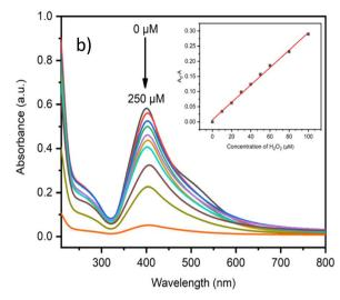
Fig. 6 (a) Absorption spectra showing (a) SPR bands of AgNPs and after addition of  $H_2O_2$  solution; inside showing the colorimetric image. (b) UV-vis absorption spectra AgNPs solution adding various concentrations of  $H_2O_2$  ions in the range o to 250  $\mu$ M. The inset image showed the linear relationship between the absorbance ratios ( $A/A_0$ ) versus  $H_2O_2$  ion concentration.
