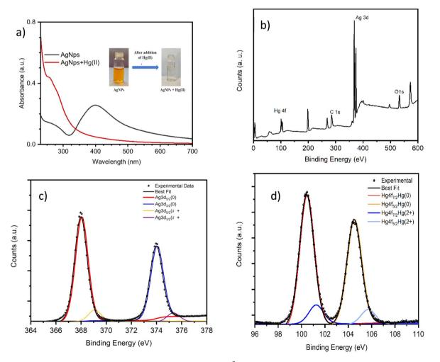
Fig. 4 Absorption spectra showing (a) SPR bands of AgNPs and AgNPs-Hg<sup>2+</sup>. Inset image showing colorimetric picture AgNPs (brown colour solution) and AgNPs-Hg<sup>2+</sup> (colourless). (b) SR-XPS survey spectra of AgNPs-Hg. (c) XPS Ag 3d core level spectra (d) XPS Hg 4f spectra.
