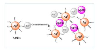
Fig. 3 Schematic representation of Ag and Hg interaction during Hg<sup>2+</sup> detection using AgNPs due to oxidation reduction reaction.
