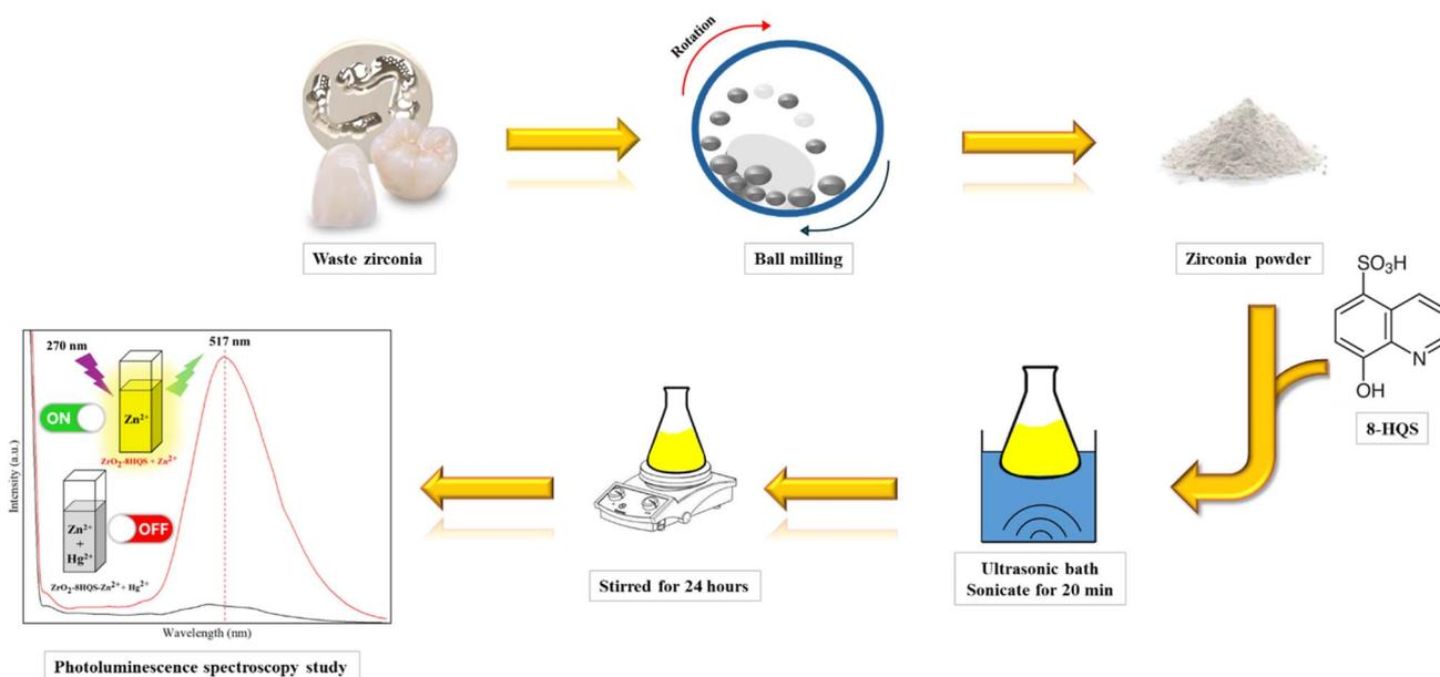
Scheme 1 Schematic of the preparation of ZrO<sub>2</sub>-8-HQS as an on-off optical chemo-probe for sensing Zn<sup>2+</sup> and Hg<sup>2+</sup>.
