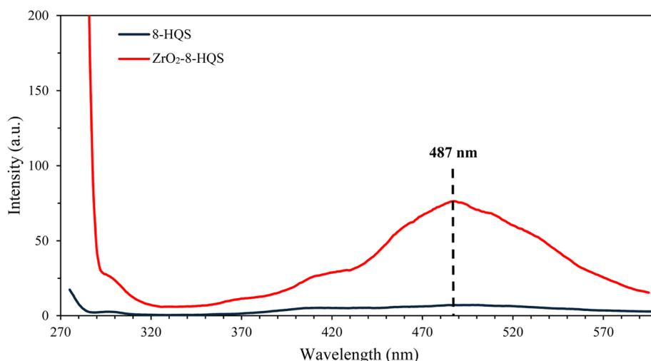
Fig. 4 Fluorescence emission comparison of 8-HQS (dark blue line) and ZrO<sub>2</sub>-8-HQS (red line) ( $\lambda_{\text{ex}} = 270$  nm).
