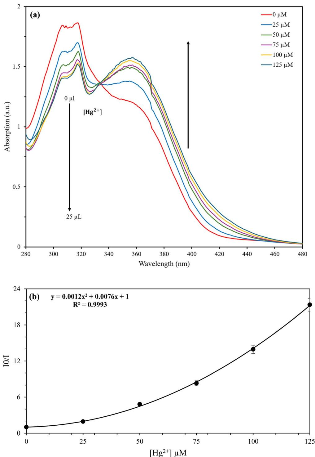
Fig. 7 (a) Titration plot of  $\text{ZrO}_2\text{-8-HQS-Zn}^{2+}$  through the addition of  $\text{Hg}^{2+}$ . (b) Non-linear modified Stern–Volmer quenching plot.
