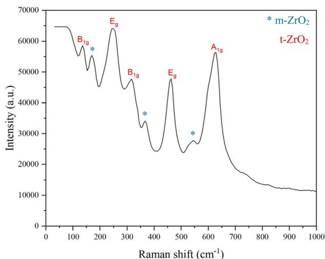
Fig. 3 Raman spectrum of ZrO<sub>2</sub> NPs prepared from WBDPs.
