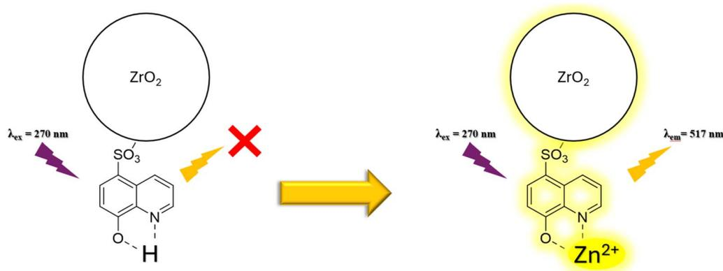
Scheme 2 Mechanistic pathway of the ZrO<sub>2</sub>-8-HQS for the sensing of Zn<sup>2+</sup>.Table 2 Compression of different studies to detect Zn<sup>2+</sup>
