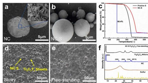
Fig. 2 SEM images of (a) NC and (b) NC-S, (c) TG curves of S and NC-S. SEM images of (d) NC-S/ $\text{Ti}_3\text{C}_2\text{T}_x$  slurry and (e) free-standing NC-S/ $\text{Ti}_3\text{C}_2\text{T}_x$  film. (f) XRD patterns of sulfur, NC,  $\text{Ti}_3\text{C}_2\text{T}_x$  MXene and free-standing NC-S/ $\text{Ti}_3\text{C}_2\text{T}_x$ .
