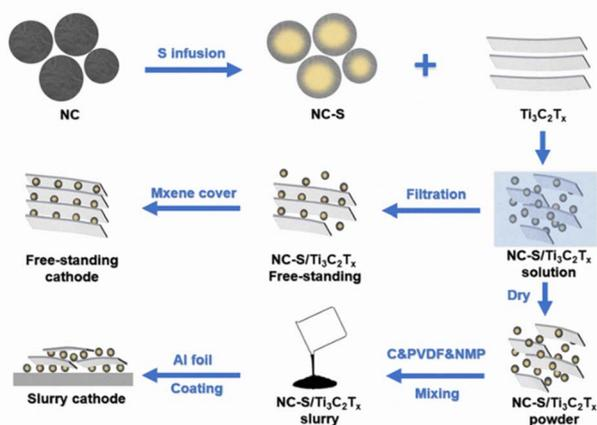
Fig. 1 Schematic of the fabrication of slurry coating and free-standing NC-S/ $\text{Ti}_3\text{C}_2\text{T}_x$  MXene hybrids.
