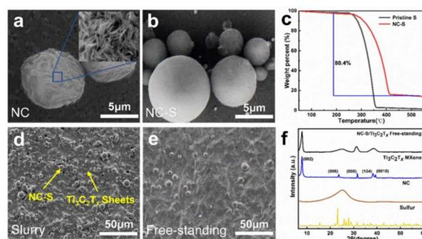
Fig. 2 SEM images of (a) NC and (b) NC-S, (c) TG curves of S and NC-S. SEM images of (d) NC-S/Ti<sub>3</sub>C<sub>2</sub>T<sub>x</sub> slurry and (e) free-standing NC-S/Ti<sub>3</sub>C<sub>2</sub>T<sub>x</sub> film. (f) XRD patterns of sulfur, NC, Ti<sub>3</sub>C<sub>2</sub>T<sub>x</sub> MXene and free-standing NC-S/Ti<sub>3</sub>C<sub>2</sub>T<sub>x</sub>.
