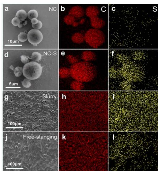
Fig. 3 SEM images and EDS mappings of C and S of (a–c) NC before sulfur infusion, (d–f) NC-S, (g–i) NC-S/Ti<sub>3</sub>C<sub>2</sub>T<sub>x</sub> slurry and (j–l) the free-standing NC-S/Ti<sub>3</sub>C<sub>2</sub>T<sub>x</sub> film.
