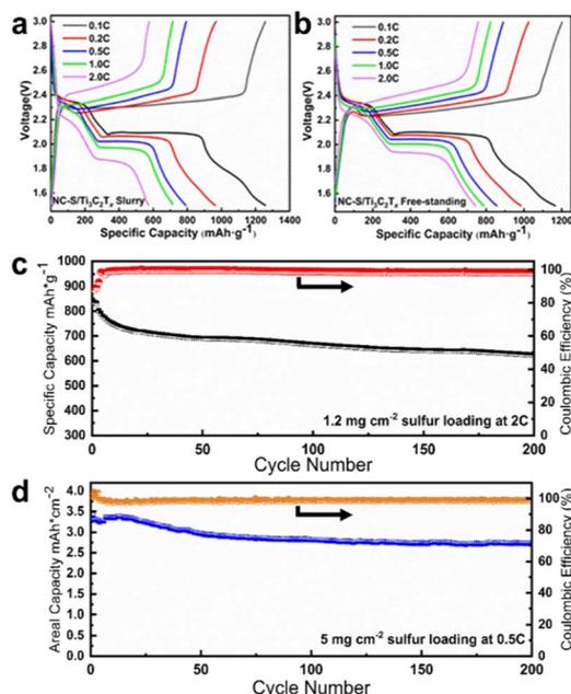
Fig. 5 First discharge and charge curves of (a) NC-S/Ti<sub>3</sub>C<sub>2</sub>T<sub>x</sub> slurry and (b) free-standing NC-S/Ti<sub>3</sub>C<sub>2</sub>T<sub>x</sub> cathodes at different rates. Cycling performance and coulombic efficiency of the free-standing NC-S/Ti<sub>3</sub>C<sub>2</sub>T<sub>x</sub> cathode-based cells (c) at 2C and (d) at 0.5C (5.0 mg cm<sup>-2</sup> sulfur loading).
