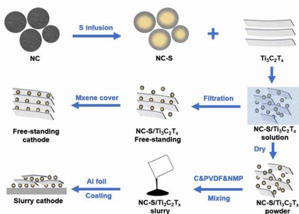
Fig. 1 Schematic of the fabrication of slurry coating and free-standing NC-S/Ti<sub>3</sub>C<sub>2</sub>T<sub>x</sub> MXene hybrids.
