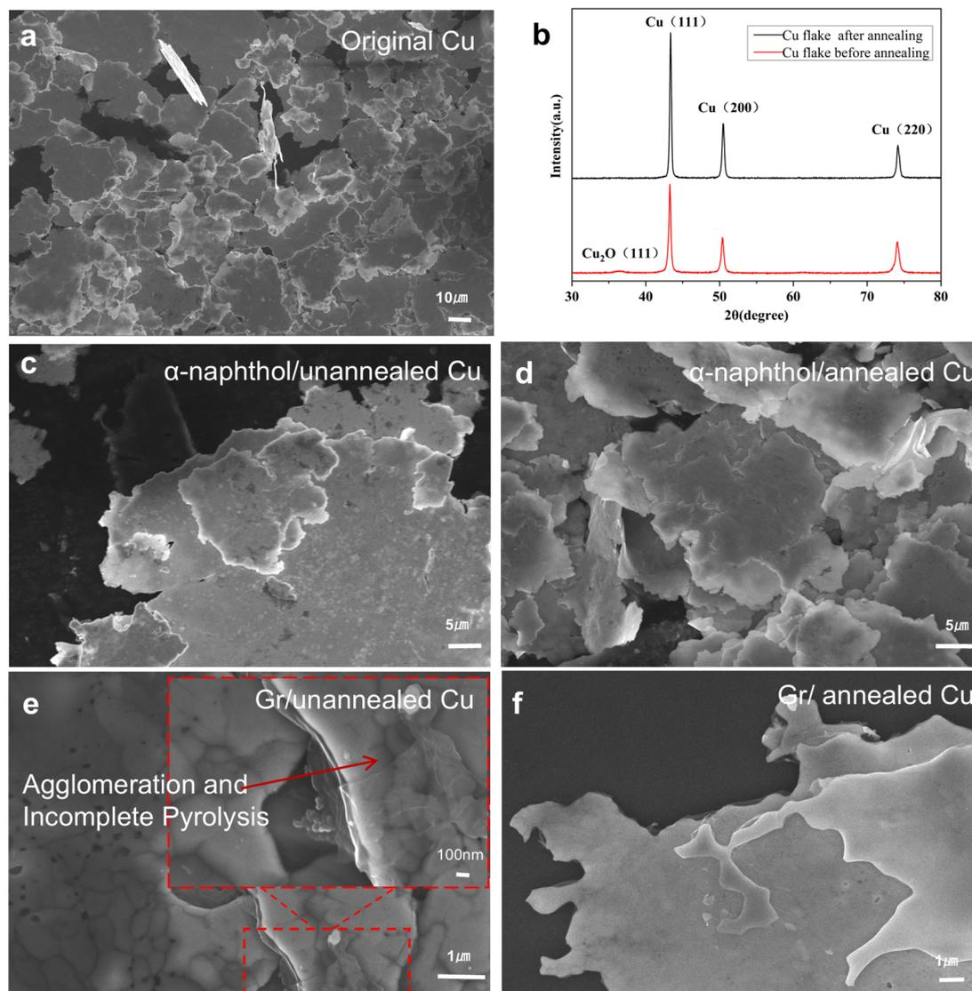
Fig. 2 (a) SEM image of the original Cu powders. (b) XRD patterns of Cu powders before and after annealing. (c)  $\alpha$ -Naphthol/unannealed Cu. (d)  $\alpha$ -Naphthol/unannealed Cu. (e) Gr/unannealed Cu. (f) Gr/annealed Cu.
