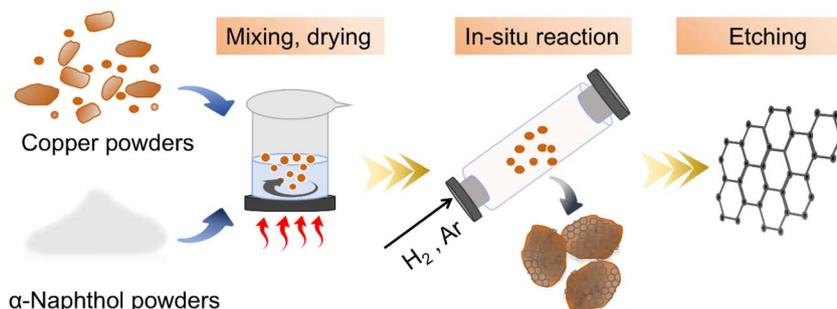
Fig. 1 Schematic of *in situ* Gr growth processes.
