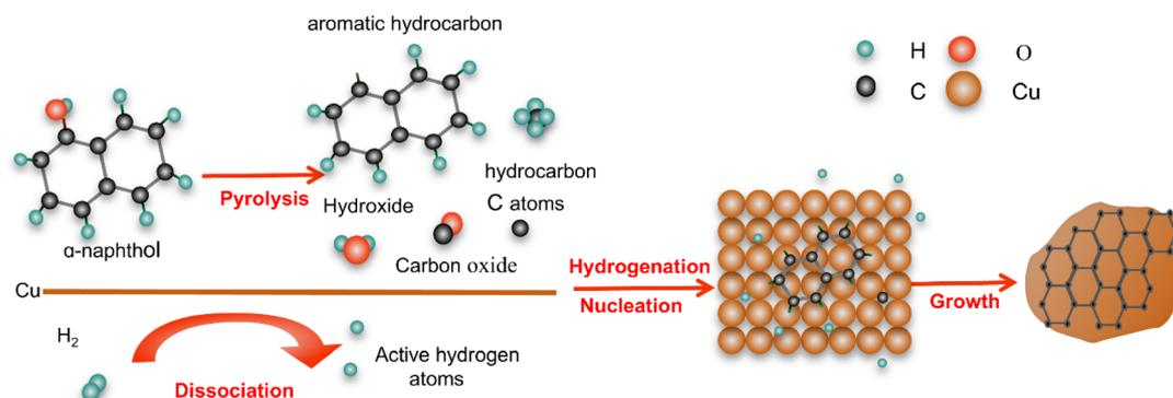
Fig. 7 A schematic to illustrate the processes involved in  $\alpha$ -naphthol based *in situ* growth of Gr on the Cu substrate.
