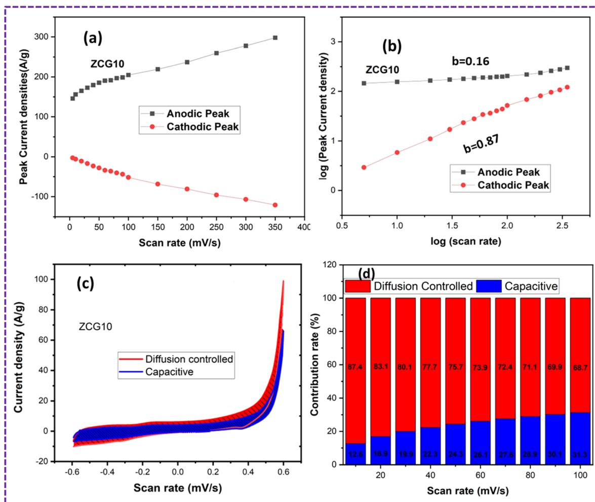
Fig. 12 Charge storage mechanism of ZCG10 nanocomposite: (a) graph between scan rate ( $\text{mV s}^{-1}$ ) and peak current density ( $\text{A g}^{-1}$ ) (b) graph between  $\log(\text{scan rate})$  and  $\log(\text{peak current density})$  (c) graph of diffusion-controlled and capacitive contribution at  $20 \text{ mV s}^{-1}$  and (d) percentage of diffusion-controlled and capacitive contribution at different scan rates.
