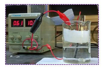
Graphene synthesis by electrochemical exfoliation.
