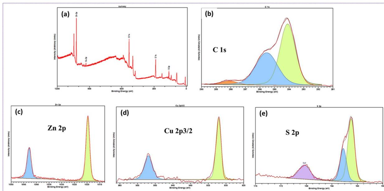
Fig. 8 (a) XPS survey spectra of ZCS10 (b) spectra of C 1s (c) spectra of Zn 2p, (d) spectra of Cu 2p<sub>3/2</sub>, (e) spectra of S 2p.
