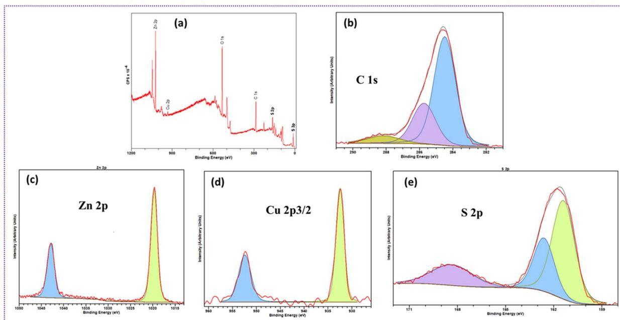
Fig. 9 (a) XPS survey spectra of ZCG10 (b) spectra of C 1s (c) spectra of Zn 2p, (d) spectra of Cu 2p<sub>3/2</sub>, (e) spectra of S 2p.
