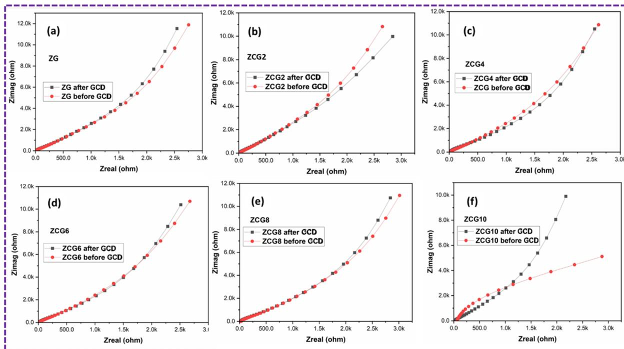
Fig. 17 Nyquist plot of (a) ZG, (b) ZCG2, (c) ZCG4, (d) ZCG6, (e) ZCG8 and (f) ZCG10 after 1000 cycles before and after GCD.
