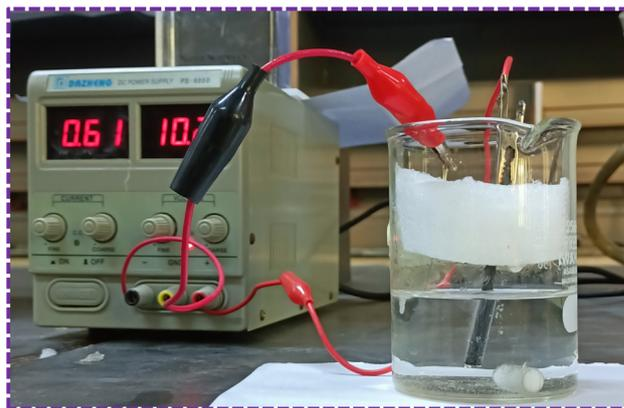
Fig. 2 Graphene synthesis by electrochemical exfoliation.
