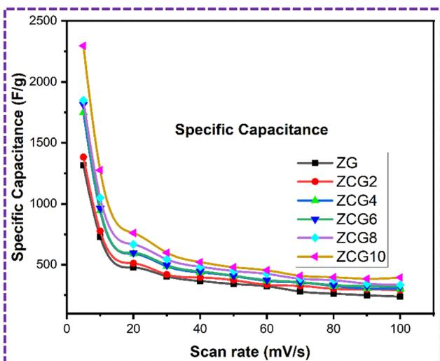
Fig. 11 Comparison of specific capacitance graph by CV.
