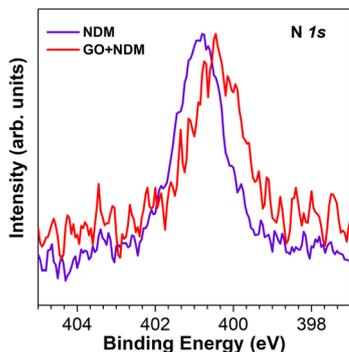
Fig. 7 Normalized N 1s XPS core-level spectra of pure NDM-1 0.5 mg ml<sup>-1</sup> (violet) and GO 0.5 mg ml<sup>-1</sup> mixed with NDM-1 0.5 mg ml<sup>-1</sup> (red).
