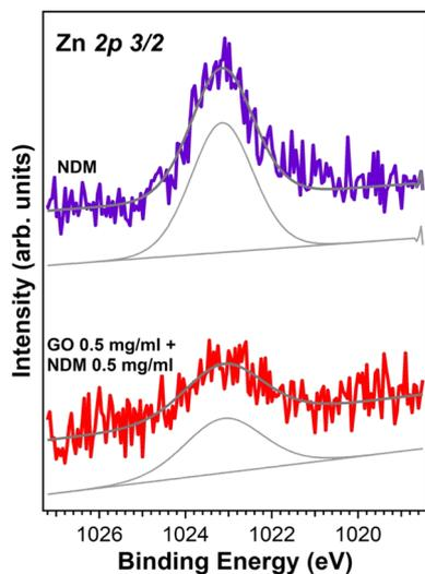
Fig. 5 Zn  $2p_{3/2}$  XPS core-level spectra for: upper curve (violet) NDM-1  $0.5 \text{ mg ml}^{-1}$  on Au/Si(100), and lower curve (red) (GO  $0.5 \text{ mg ml}^{-1}$  + NDM-1  $0.5 \text{ mg ml}^{-1}$ ) on Au/Si(100). Fitting and background curves are reported in light grey.
