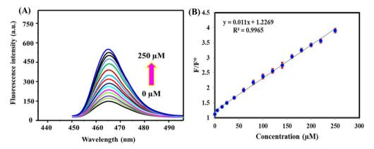
Fig. 4 (A) The FL signal spectra of PEI/DTH@NiNCs Fe<sup>3+</sup> system after addition of GSH in the range of 0 to 250 μM. (B) Calibration plot between F/  $F^0$  and concentration of GSH.
