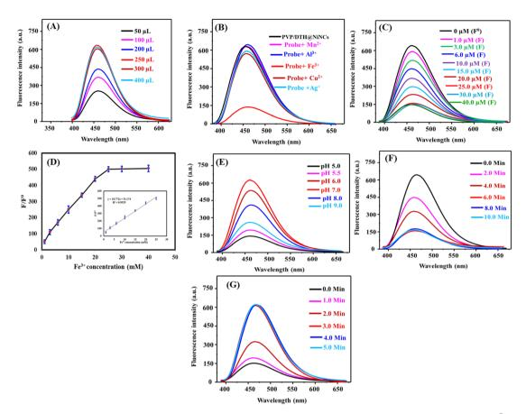
Fig. 3 Influence of the detection parameters: (A) volume of PEI/DTH@NiNCs, (B) different metal ions (25.0  $\mu$ M), (C) different Fe<sup>3+</sup> concentration (0–40  $\mu$ M), (D) calibration plot between  $F/F^0$  and concentration of Fe<sup>3+</sup> ion, (E) pH value, (F) reaction time between PEI/DTH@NiNCs and 25.0  $\mu$ M Fe<sup>3+</sup> ion, (G) reaction time between PEI/DTH@NiNCs/Fe<sup>3+</sup> and GSH.
