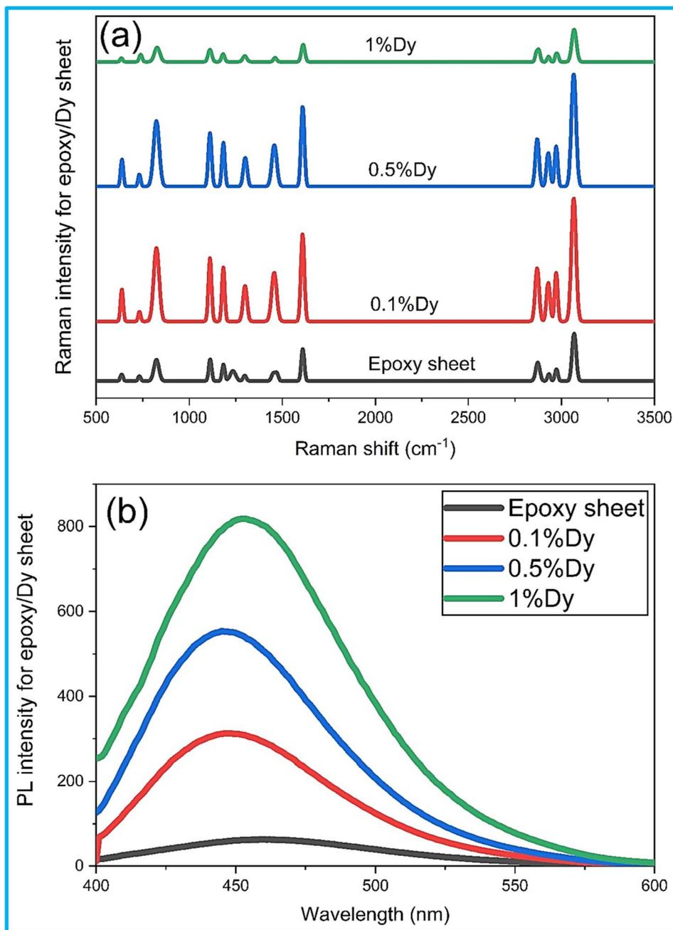
Fig. 5 Characterization of pristine epoxy sheets containing different concentrations of Dy ions: (a) Raman spectra of epoxy/Dy sheets and (b) PL emission spectra of epoxy/Dy sheets.
