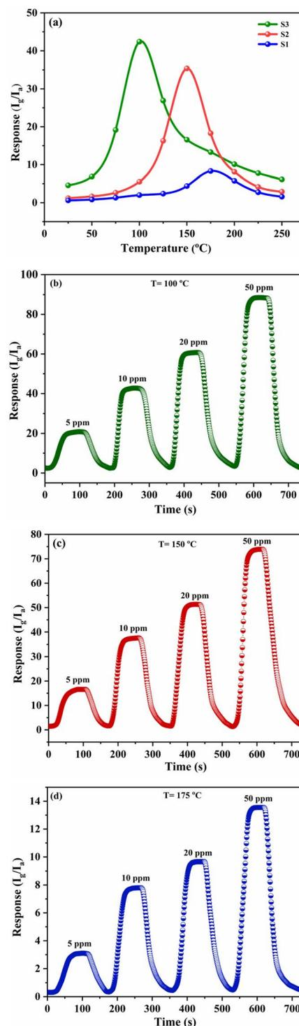
Fig. 8 (a) The gas-sensing performance of the S1, S2 and S3 sensors toward 10 ppm H<sub>2</sub>S at various temperatures, (b)–(d) gas sensing curves for H<sub>2</sub>S concentrations ranging from 5 ppm to 50 ppm, for S3, S2 and S1 gas sensors at 100 °C, 150 °C and 175 °C.
