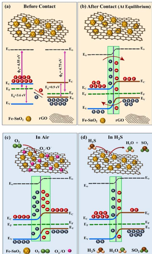
Fig. 12 Gas sensing mechanism of S3 nanocomposite sensor in (a) energy band diagram of Fe–SnO<sub>2</sub> and rGO before contact (b) after contact (at equilibrium) (c) air (d) H<sub>2</sub>S.
