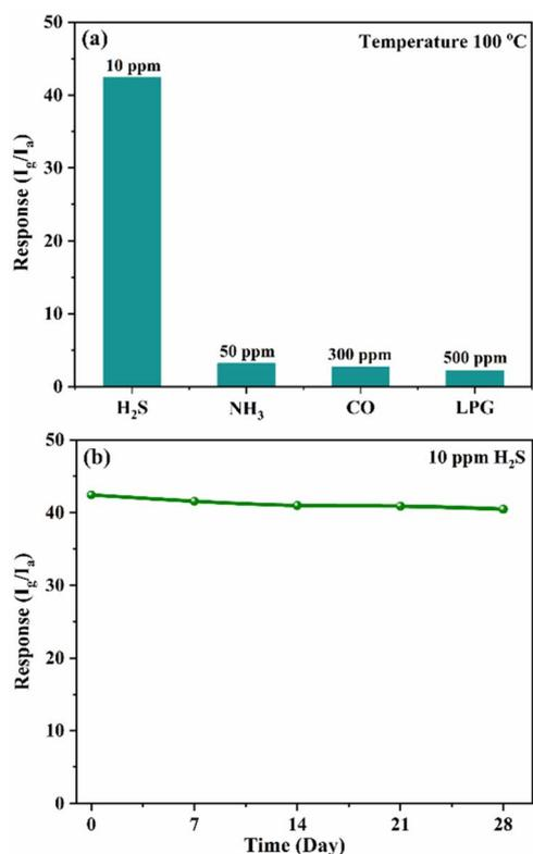
Fig. 11 (a) Selectivity of S3 nanocomposite sensor towards NH<sub>3</sub> (50 ppm), CO<sub>2</sub> (300) and LPG (500 ppm) at 100 °C, (b) long term stability of S3 nanocomposite sensor.
