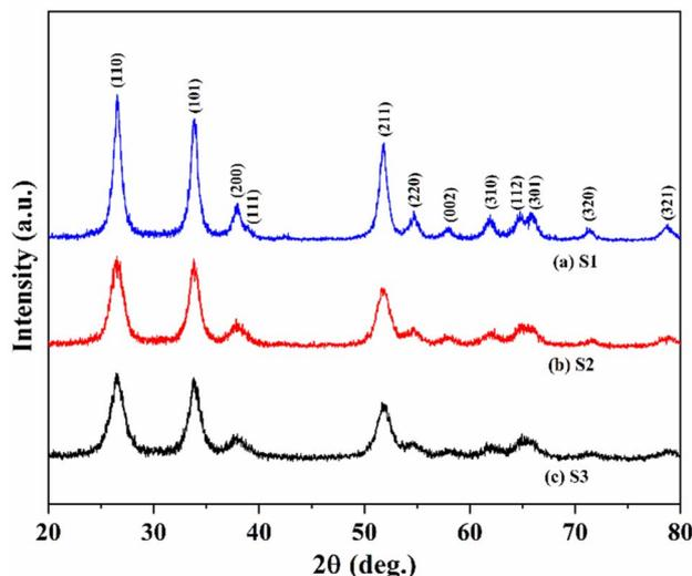
Fig. 1 X-ray diffraction pattern of samples (a) S1 (b) S2 and (c) S3 respectively.
