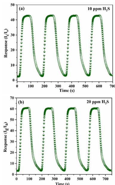
Fig. 10 Repeatability of S3 sensor to (a) 10 ppm and (b) 20 ppm  $\text{H}_2\text{S}$  at 100 °C.
