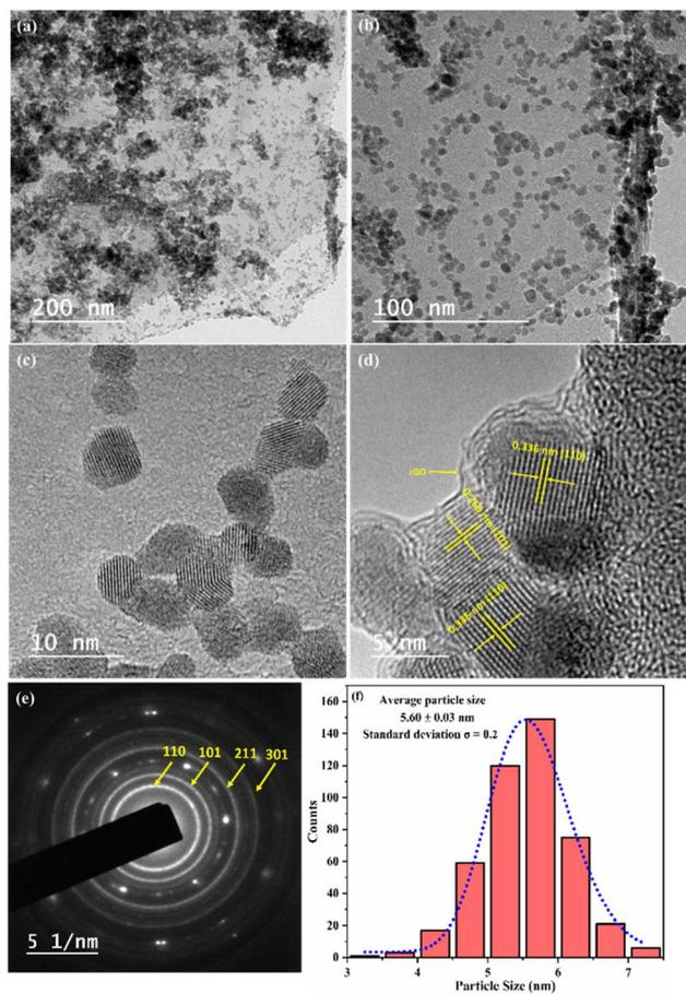
Fig. 2 (a–d) Low and high resolution HR-TEM micrographs (e) SAED pattern and (f) particle size histogram of S3 nanocomposite.
