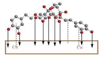
Fig. 4 Schematic illustration of inhibition mechanism of ACT adsorption on copper in 1.0 M  $\rm HNO_3$  yielding the formation of protective layer.
