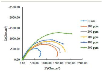
Fig. 6 Nyquist plots for Cu corrosion at 303 K using the investigated inhibitor ACT and in a 1.0 M HNO<sub>3</sub> solution.
