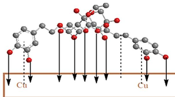
Fig. 4 Schematic illustration of inhibition mechanism of ACT adsorption on copper in 1.0 M HNO<sub>3</sub> yielding the formation of protective layer.
