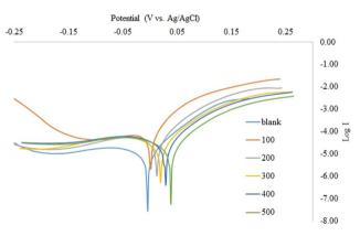
Fig. 5 Copper polarization anodic and cathodic curves in  $1.0 \text{ M HNO}_3$  with and without different ACT concentrations.
