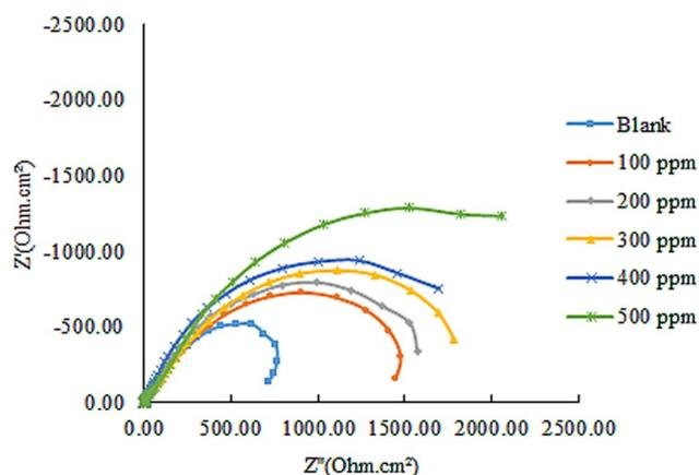
Fig. 6 Nyquist plots for Cu corrosion at 303 K using the investigated inhibitor ACT and in a 1.0 M HNO<sub>3</sub> solution.
