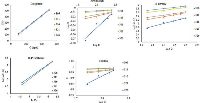
Fig. 3 Adsorption isotherms for copper specimen with ACT in 1.0 M HNO<sub>3</sub> for 4 h at different temperatures.
