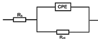
Fig. 7 The EIS data for Cu corrosion in 1.0 M HNO<sub>3</sub> solution and with the investigated inhibitor ACT were fitted using an electrochemical equivalent circuit.
