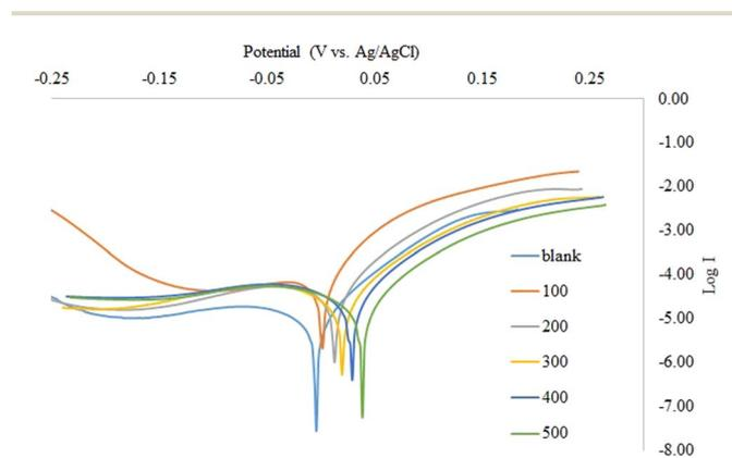
Fig. 5 Copper polarization anodic and cathodic curves in 1.0 M  $\text{HNO}_3$  with and without different ACT concentrations.
