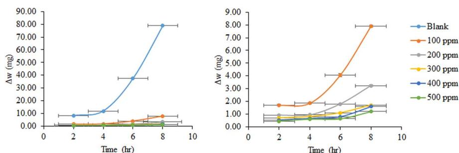
Fig. 2 Weight loss–time curves for copper corrosion in 1.0 M HNO<sub>3</sub> at 28 °C with and without varying ACT concentrations.
