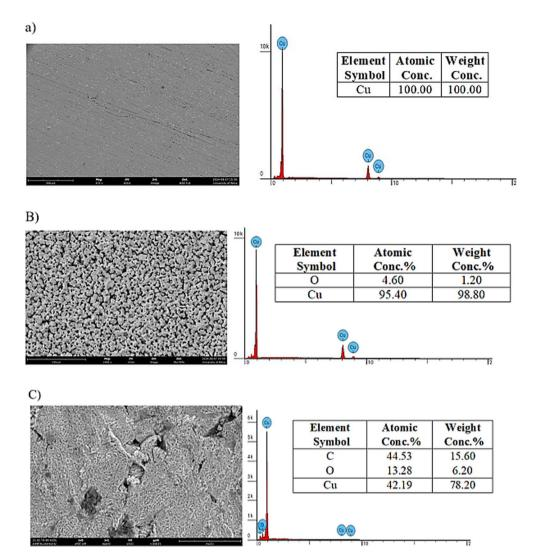
Fig. 8 SEM image and EDS mapping of copper surface (A) without immersion (B) in 1.0 M HNO $_3$  (C) presence of 300 ppm of ACT.
