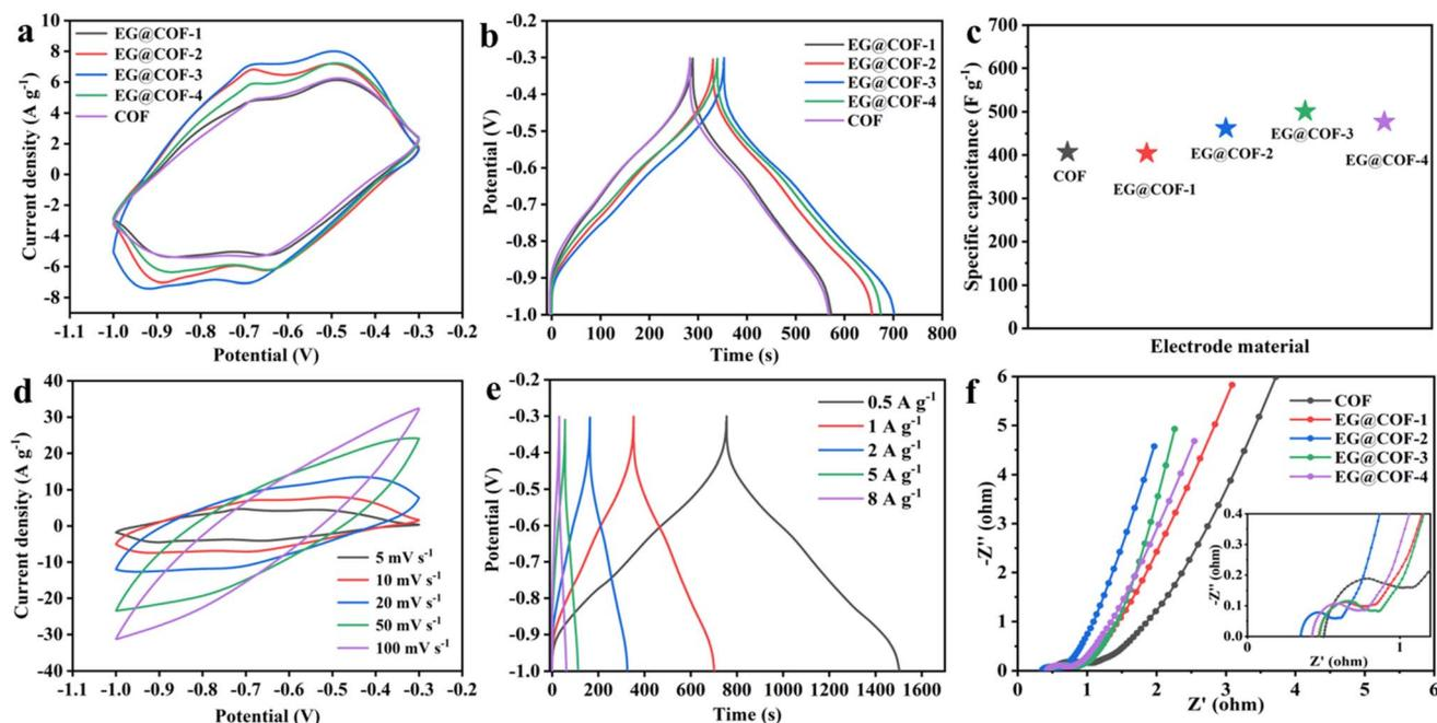
Fig. 4 (a) Comparison of cyclic voltammetry (CV) curves of EG@COFs and pure COF at a scan rate of  $10 \text{ mV s}^{-1}$ , (b) GCD curves of EG@COFs and pure COF at different current densities, (c) comparison of specific capacitance values of different materials in this work, (d) CV curves of EG@COF-3 with different scan rates, (e) GCD curves of EG@COF-3 with different current densities, (f) electrochemical impedance spectra of EG@COFs and pure COF.
