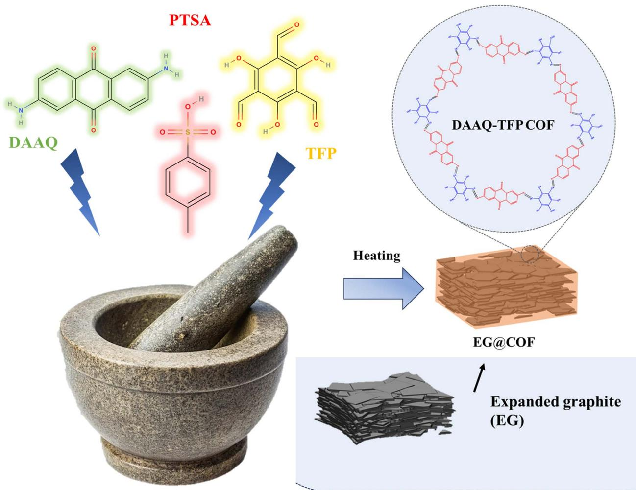
Scheme 1 Schematic of the synthesis of EG@COF.
