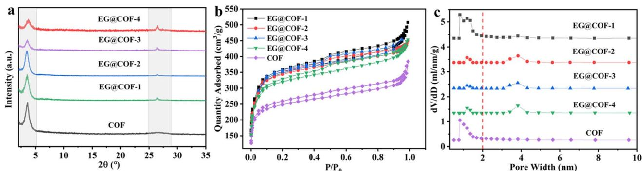
Fig. 1 (a) Powder X-ray diffraction patterns of pure COF and EG@COFs, (b) N<sub>2</sub> adsorption and desorption isotherms recorded at 77 K, (c) pore size distributions of pristine COF and EG@COFs calculated from the adsorption isotherms.
