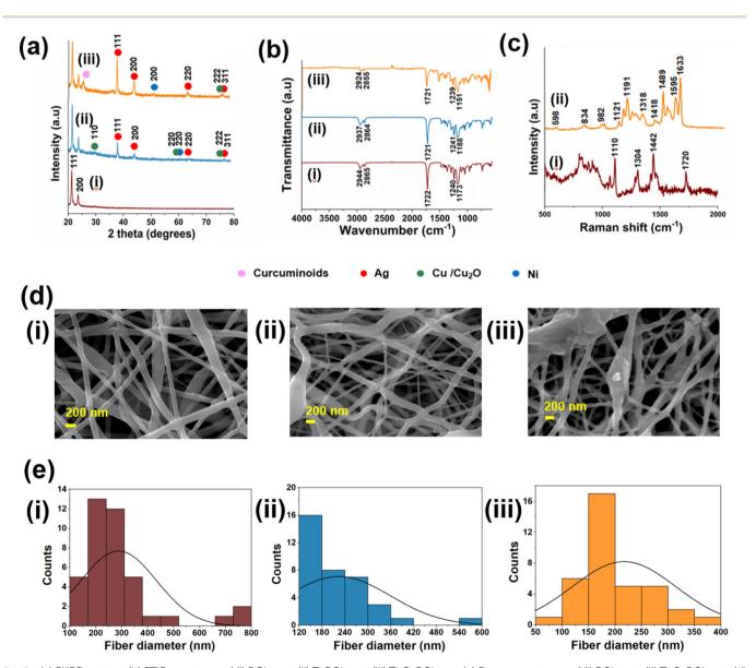
Fig. 3 (a) PXRD pattern (b) FTIR spectrum of (i) PCL mat, (ii) T-PCL mat (iii) T-C-PCL mat (c) Raman spectrum of (i) PCL mat, (ii) T-C-PCL mat (d) SEM images (e) fiber diameter distribution of (i) PCL mat, (ii) T-PCL mat, and (iii)T-C-PCL mat.
