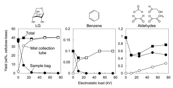
Fig. 6 Yields of LG, benzene and aldehydes at various electrostatic loads (■: total yield, O: yield in mist collection tube, •: yield in sample bag).
