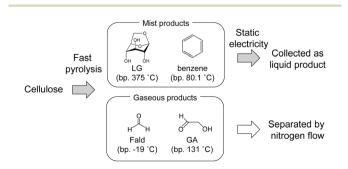
Fig. 7 The effect of static electricity on the pyrolysis products of cellulose in fast pyrolysis under infrared irradiation.
