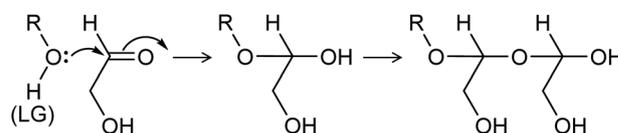
Fig. 5 Acetalization of the OH of LG with the aldehyde group of GA.
