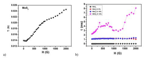
Fig. 9 Variation in relaxation time with respect to magnetic field at room temperature for (a)  $MoS_2$  and  $MoS_2$  nanoparticles doped with (b) 5%, 10% and 15% Cr.
