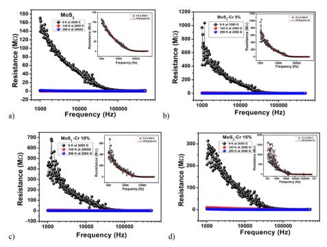
Fig. 13 Variation of resistance with respect to frequency at various temperatures and an applied magnetic field of 2000 G for (a)  $MoS_2$  and  $MoS_2$  nanoparticles doped with (b) 5%, (c) 10% and (d) 15% Cr.
