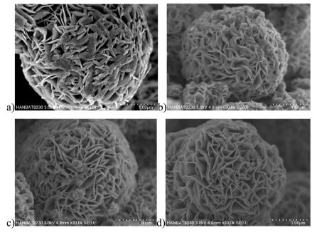
Fig. 2 SEM images of (a) pure MoS<sub>2</sub> nanoparticles and those doped with (b) 5% Cr, (c) 10% Cr, and (d) 15% Cr.
