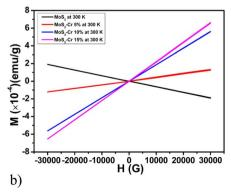
Hysteresis loop for MoS<sub>2</sub> and MoS<sub>2</sub> nanoparticles doped with 5%, 10% and 15% Cr at (a) 10 K and (b) 300 K.
