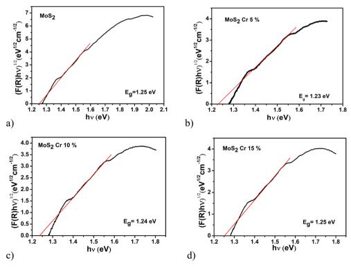
Fig. 4 Indirect bandgap of (a) pure MoS<sub>2</sub> nanoparticles and those doped with (b) 5% Cr, (c) 10% Cr, and (d) 15% Cr.
