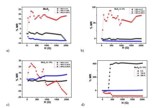
Fig. 15 Variation of AC magnetoresistance with respect to an applied magnetic field at a frequency of 1 MHz for (a)  $MoS_2$  and  $MoS_2$  nanoparticles doped with (b) 5% Cr, (c) 10% Cr and (d) 15% Cr.
