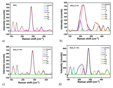
Fig. 5 Raman spectra of (a) MoS<sub>2</sub> and MoS<sub>2</sub> nanoparticles doped with (b) 5% Cr, (c) 10% Cr, and (d) 15% Cr.
