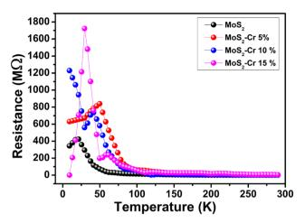
Fig. 11 Variation of resistance with respect to temperature at a frequency of 100 Hz.
