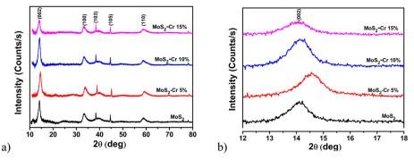
Fig. 1 (a) XRD patterns of pure  $MoS_2$  nanoparticles and those doped with 5%, 10% and 15% Cr. (b) Peak shift with respect to the variation in doping percentage of chromium.
