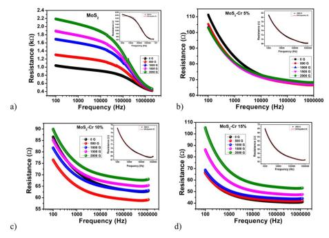
Fig. 8 Variation of resistance with respect to frequency in the presence of a magnetic field for (a) MoS<sub>2</sub> and MoS<sub>2</sub> nanoparticles doped with (b) 5% Cr, (c) 10% Cr, and (d) 15% Cr.
