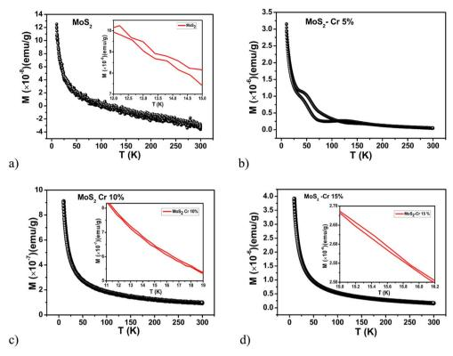
Fig. 7 M-T for (a) pure MoS<sub>2</sub> nanoparticles and those doped with (b) 5% Cr, (c) 10% Cr, and (d) 15% Cr.
