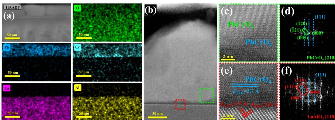
Fig. 2 (a) EDS mapping of each element of the  $\text{PbCrO}_4/\text{LAO}$  thin film. (b) Cross-sectional image of the sample. (c and e) HRTEM images and (d and f) FFT transformation images of the green and red rectangles in (b), respectively.
