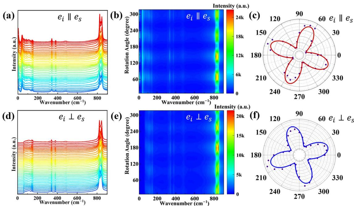
Fig. 4 ARPRS spectra of PbCrO<sub>4</sub>/LAO thin films under (a) horizontal and (d) vertical scattering geometries. (b and e) Contour color maps of ARPRS results. Raman polarization fitting diagram of the 823 cm<sup>-1</sup> mode under (c) horizontal and (f) vertical configurations.
