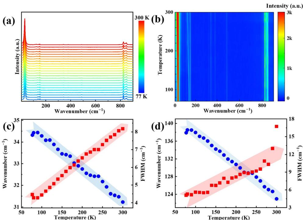
Fig. 5 (a) Temperature-dependent Raman spectroscopy of the PbCrO<sub>4</sub>/LAO thin film. (b) Contour color map. Peak positions (blue) and FWHM (red) vary with temperature for (c) 34 cm<sup>-1</sup> and (d) 138 cm<sup>-1</sup>, respectively.
