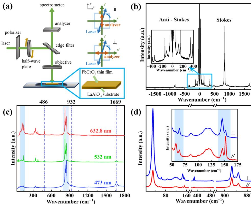
Fig. 3 (a) Schematic diagram of the ARPRS of the  $\text{PbCrO}_4$  thin film. (b) Stokes and anti-Stokes curves of  $\text{PbCrO}_4$ . Inset: magnified view at ultra-low frequency. (c) Multi-wavelength Raman spectra of the  $\text{PbCrO}_4$  thin film. (d) Typical Raman spectra under horizontal and vertical polarization. Inset: magnified view from 50 to  $175 \text{ cm}^{-1}$ .
