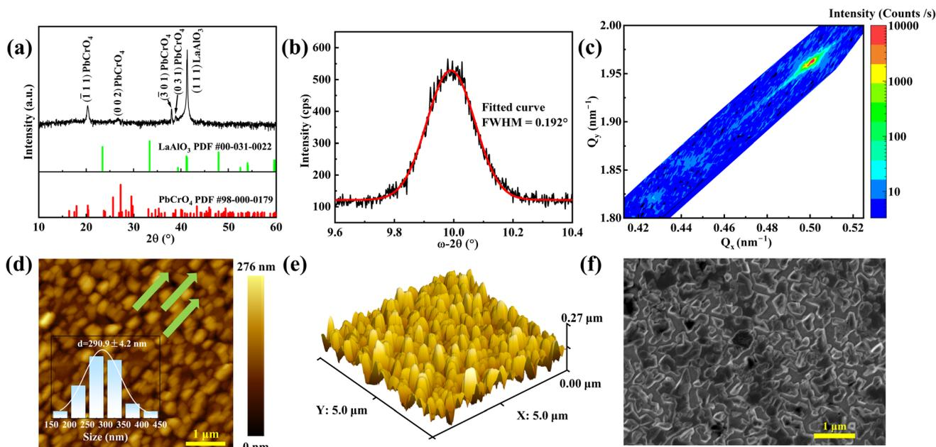
Fig. 1 (a) Experimental powder XRD pattern. Here, the red and green lines denote the standard peaks of  $\text{PbCrO}_4$  and LAO, respectively. (b) Rocking curve of (111), and (c) RSM image of the  $\text{PbCrO}_4/\text{LAO}$  thin film. (d) Two-dimensional (2D) and (e) three-dimensional (3D) AFM images of the sample. Inset: grain size profile. (f) SEM image of the  $\text{PbCrO}_4/\text{LAO}$  thin film.
