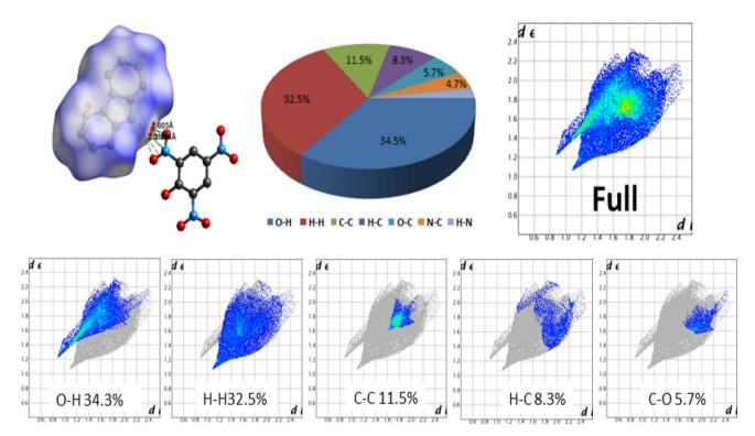
Fig. 3 In a  $d_{\text{norm}}$  surface, red spots show strong hydrogen bonds between acceptor and donor atoms, white light red spots indicate weak intermolecular interactions. The  $d_{\text{norm}}$  plots were plotted with a color scale between blue and red from -0.376 to 1.134.
