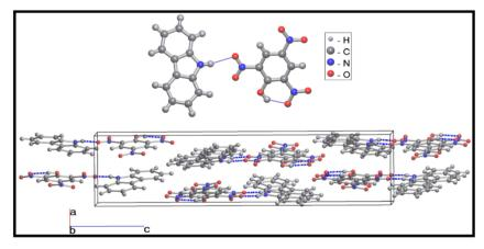
Fig. 2 The hydrogen-bonded dimer of carbazole and picric acid (top) and the packing of the dimers in the unit cell (bottom). The hydrogen bonds are highlighted in blue.
