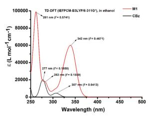
Fig. 5 Theoretical UV-Vis absorption spectra for M1 and CBz.
