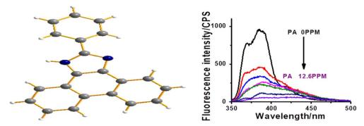
Fig. 12 Molecular structure of M1 and its fluorescence guenching with PA
