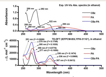
Fig. 4 Comparison of UV-Vis absorption spectra of CBz-PA, recorded in EtOH (1 imes 10<sup>-4</sup> M), with the spectra ( $\varepsilon$ -molar absorptivity, f-oscillator strength) obtained from TD-DFT calculations in solution phase.
