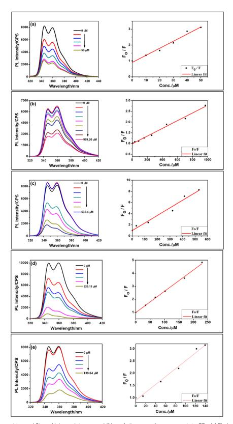
Fig. 11 Fluorescence quenching and Stern-Volmer plots upon addition of nitroaromatic compounds to CBz. (a) Picric acid, (b) 1,4 dichloro-2-nitro benzene, (c) 2-nitro-aniline, (d) 4-nitro-aniline, (e) 4-nitrophenol.
