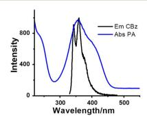
$\begin{tabular}{ll} Fig. 14 & Overlap of photoluminescence spectra of CBz and absorption spectra of PA. \end{tabular}$
