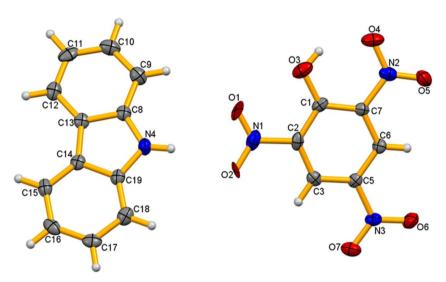
Fig. 1 Ortep view of the co-crystal CBz-PA.
