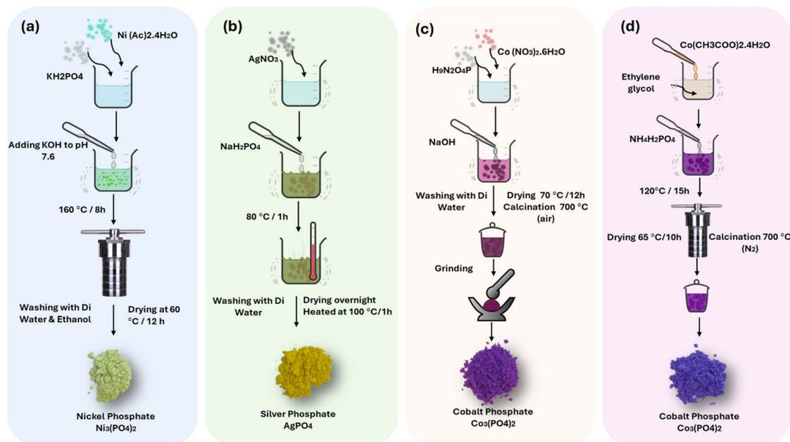
Fig. 1 Schematic illustration of the as-synthesized particles using different methods (a) Ni–P, (b) Ag–P, (c) Co–P and (d) Co–Pn.
