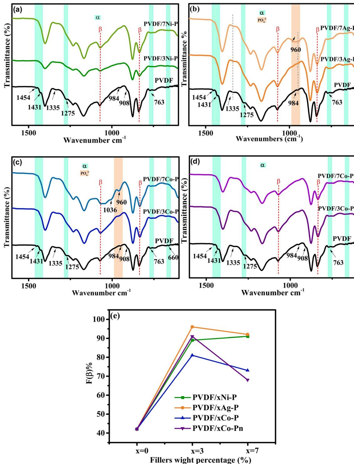
Fig. 9 FTIR spectrum (a)–(d) along with  $\beta$ -phase percentage (e) of the elaborate composite films.
