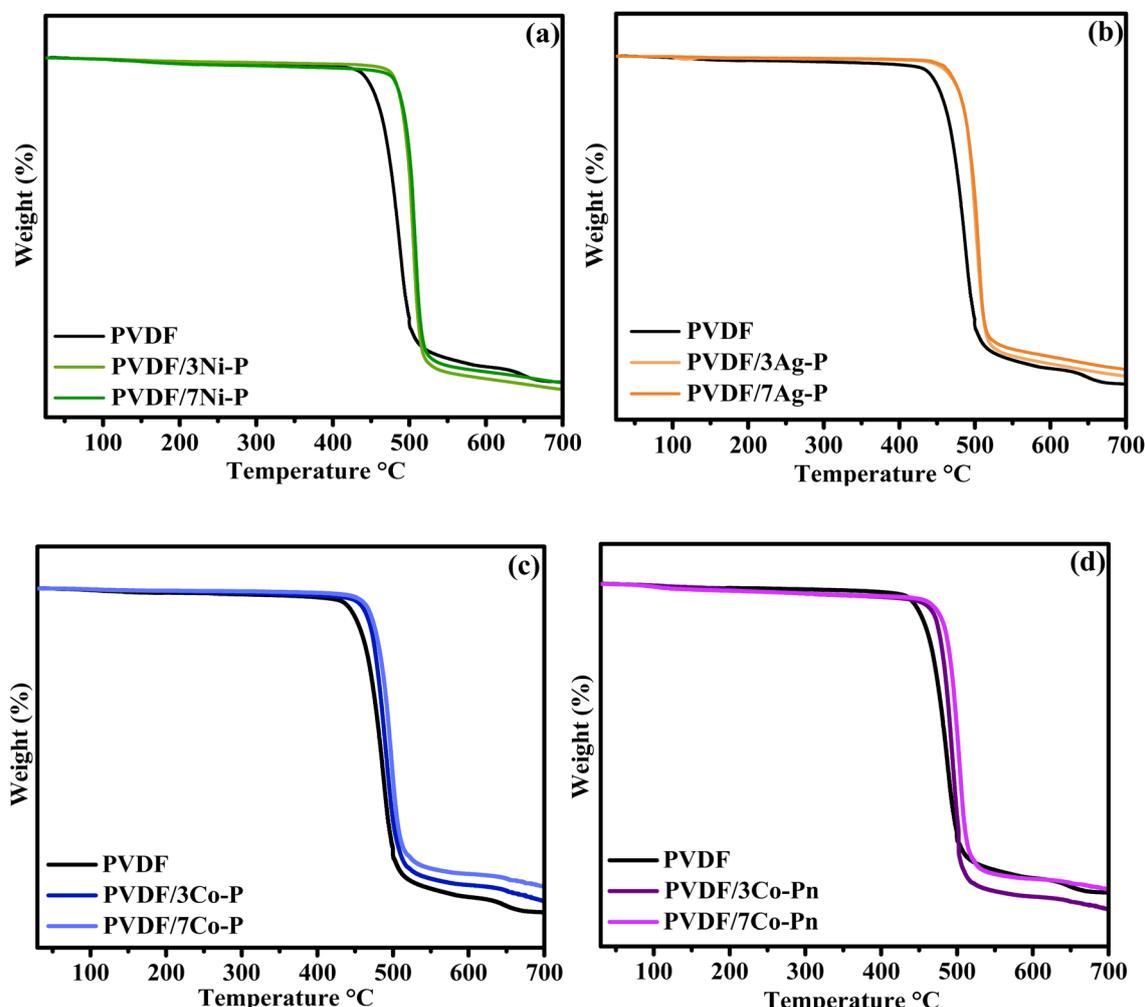
Fig. 11 TGA curves of PVDF and composite films (a) PVDF/Ni–P, (b) PVDF/Ag–P, (c) PVDF/Co–P and (d) PVDF/Co–Pn.
