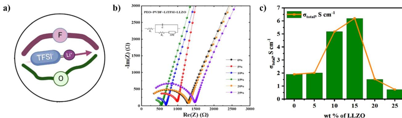
Fig. 2 (a) Schematic ion transport pathways diagram within composite electrolyte; (b) EIS results for spin-coated composite thin-film electrolytes PEO/PVDF/LiTFSI/LLZO at room temperature; (c) ionic conductivity dependence of composite thin-film solid electrolyte on LLZO concentration in polymer matrix.
