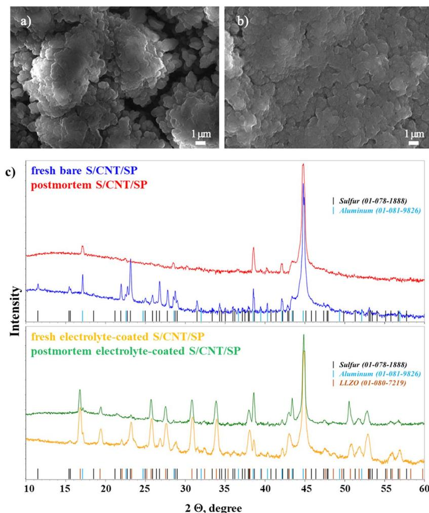
Fig. 5 Results of *post-mortem* analysis of electrodes after 150 cycles: (a) bare S/CNT/SP electrode; (b) S electrode with PEO/PVDF/LiTFSI/LLZO; (c) XRD spectra of bare and electrolyte-coated S/CNT/SP electrodes before and after cycling.
