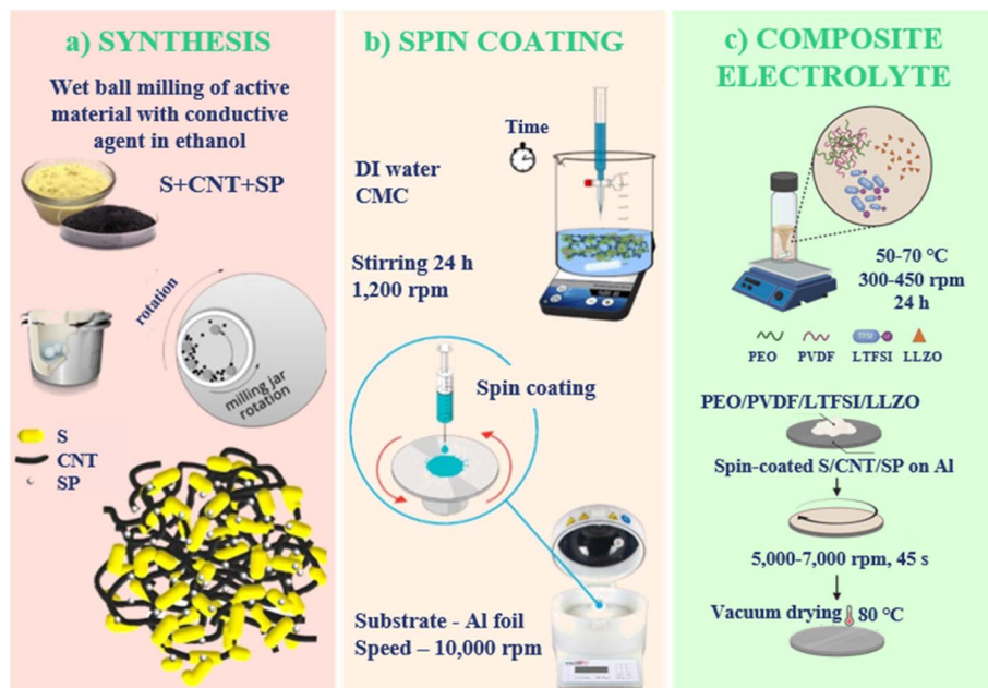
Fig. 1 Fabrication process of spin-coated S/CNT/SP cathode: (a) wet ball milling of sulfur, CNT, and Super P to achieve a well-dispersed active material mixture; (b) spin-coating of cathode slurry onto Al foil substrate; (c) schematic illustration of preparation of PEO/PVDF/LiTFSI/LLZO composite electrolyte layer by stirring polymer and ceramic components to achieve a homogeneous electrolyte mixture and its spin-coating onto Al foil with a pre-coated S/CNT/SP cathode, followed by vacuum drying at 80 °C.
