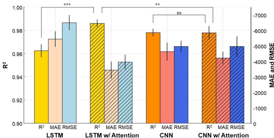
Fig. 8 Performance comparison of fatigue life prediction models (LSTM, LSTM with attention, CNN, and CNN with attention) based on  $R^2$ , MAE, and RMSE metrics. Error bars represent the standard deviation calculated from the results of the 5 model training iterations (statistically significant differences are indicated with star annotations \* $p < 0.1$ , \*\* $p < 0.05$ , and \*\*\* $p < 0.01$ ).
