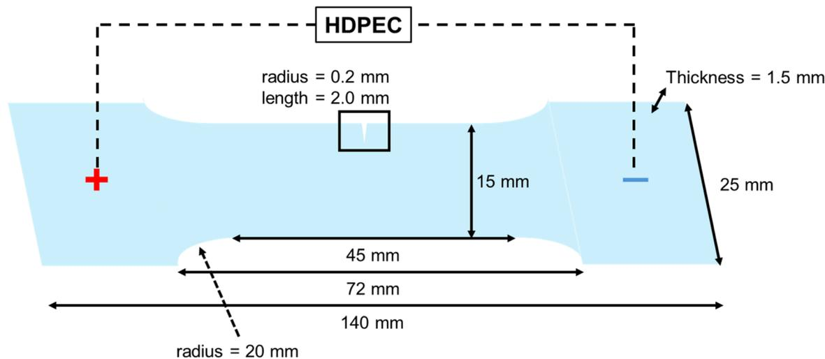
Fig. 1 Three-dimensional schematic showing the geometry of the specimens.
