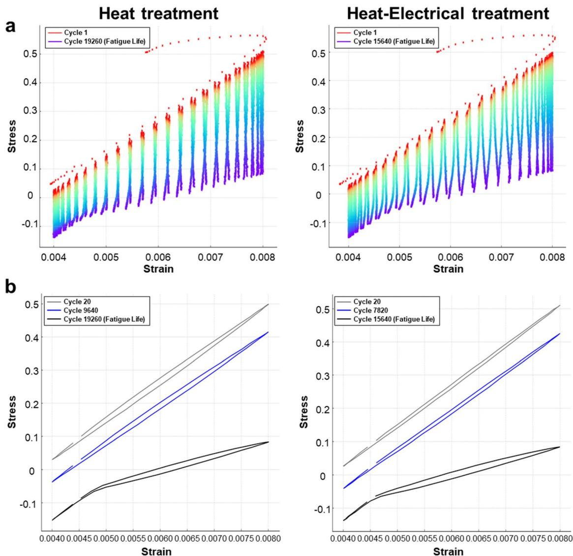
Fig. 4 Stress–strain behavior over cycles for type 316 stainless steel. (a) Stress–strain hysteresis loops for cycles at the beginning (cycle 1) and near fatigue life (cycle 19 260 and cycle 15 640). (b) Stress–strain envelope curves at intermediate cycles (cycle 7820, cycle 9640) and at fatigue life (cycle 19 260, cycle 15 640).
