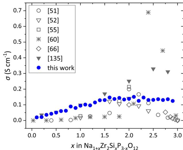
Fig. 2 Comparison of Na<sup>+</sup> conductivity of Na<sub>1+x</sub>Zr<sub>2</sub>Si<sub>x</sub>P<sub>3-x</sub>O<sub>12</sub> (0 ≤ x ≤ 3) at 598 K obtained by FFMD simulations using FF parameters derived from the CS optimization in the Na<sub>3</sub>ScZrSiP<sub>2</sub>O<sub>12</sub> training system with literature data obtained from experimental studies<sup>51,52,55,66</sup> and KMC simulations<sup>60,135</sup> at 573 K.
