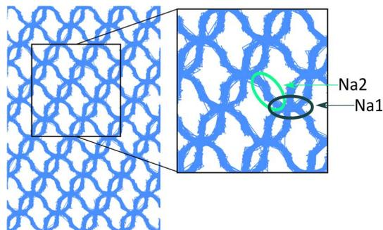
Fig. 3 The density plot of the accumulated trajectories of Na<sup>+</sup> ions in Na<sub>3</sub>Sc<sub>1.5</sub>Zr<sub>0.5</sub>Si<sub>0.3</sub>P<sub>2.7</sub>O<sub>12</sub> over the MD simulation time. The close-up view shows the well-connected diffusion pathways between the Na1 (light green) and the Na2 (dark green) sites.
