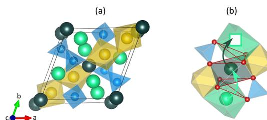
Fig. 1 (a) The primitive rhombohedral structure of NaSICONs with composition Na<sub>1+x</sub>Zr<sub>2</sub>Si<sub>x</sub>P<sub>3-x</sub>O<sub>12</sub>. (b) The correlated Na<sup>+</sup> pushing-out conduction mechanism, indicated by arrows. One Na2 ion jumps onto an occupied Na1 site pushing the Na1 ion onto an adjacent unoccupied Na2 site. Key: Na1 (dark green), Na2 (light green), ZrO<sub>6</sub> (yellow), PO<sub>4</sub>/SiO<sub>4</sub> (blue).
