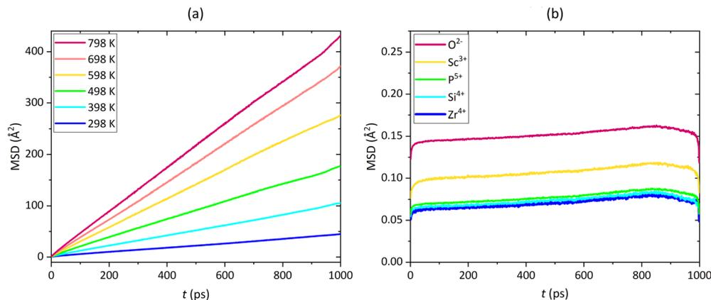
Fig. 4 MSD of (a)  $\text{Na}^+$  in the temperature range of  $298 \leq T/K \leq 798$  and (b)  $\text{O}^{2-}$ ,  $\text{Sc}^{3+}$ ,  $\text{Zr}^{4+}$ ,  $\text{Si}^{4+}$ ,  $\text{P}^{5+}$  at 698 K in  $\text{Na}_3\text{Sc}_{1.5}\text{Zr}_{0.5}\text{Si}_{0.5}\text{P}_{2.5}\text{O}_{12}$ .
