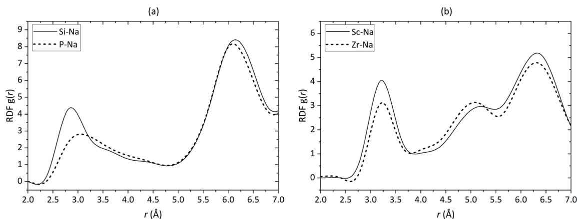
Fig. 6 Comparison of (a) RDFs of  $\text{Si}^{4+}$ - $\text{Na}^+$  (solid line) and  $\text{P}^{5+}$ - $\text{Na}^+$  (dashed line) in  $\text{Na}_{1.5}\text{Zr}_2\text{Si}_{0.5}\text{P}_{2.5}\text{O}_{12}$  and (b) RDFs of  $\text{Sc}^{3+}$ - $\text{Na}^+$  (solid line) and  $\text{Zr}^{4+}$ - $\text{Na}^+$  (dash line) in  $\text{Na}_{1.3}\text{Sc}_{0.3}\text{Zr}_{1.7}\text{P}_3\text{O}_{12}$ .
