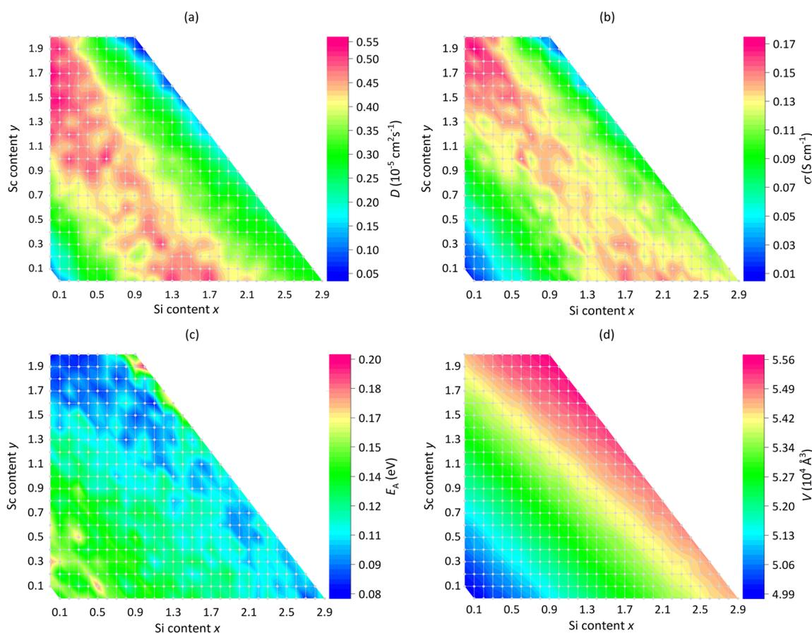
Fig. 5 (a)  $\text{Na}^+$  tracer diffusion coefficient  $D$  at 598 K, (b)  $\text{Na}^+$  conductivity  $\sigma$  obtained at 598 K, (c) activation energy  $E_A$  obtained from  $D$  at temperatures between  $498 \leq T/K \leq 798$ , and (d) cell volume  $V$  as a function of the  $\text{Sc}^{3+}$ -content  $y$  and  $\text{Si}^{4+}$ -content  $x$  in  $\text{Na}_{1+x+y}\text{Zr}_{2-y}\text{Sc}_y\text{Si}_x\text{P}_{3-x}\text{O}_{12}$ .
