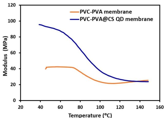
Fig. 7 The storage modulus of PVC-PVA and PVC-PVA@CS QD membranes as a function of temperature.
