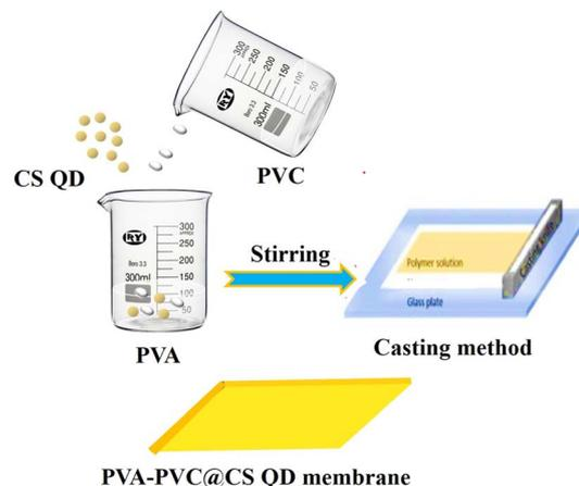
Scheme 1 Schematic diagram representing the PVA-PVC@CS QD membrane synthesis steps.
