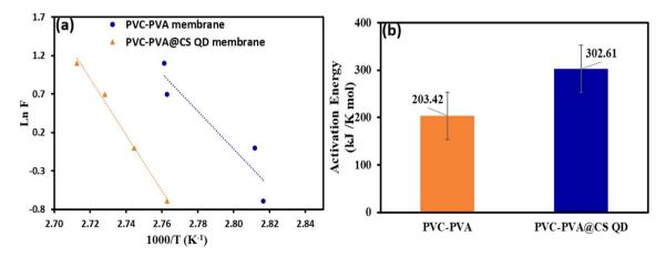
Fig. 10 (a and b): (a) The plot of ln F vs. 1000/T (K<sup>-1</sup>), and (b) the activation energy of PVC-PVA and PVC-PVA@CS QD membranes.
