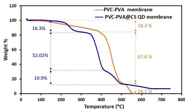
Fig. 11 The TGA of PVC-PVA and PVC-PVA@CS QD membranes.
