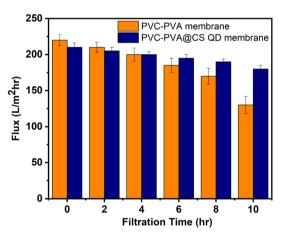
Fig. 3 Flux decline profile for PVC-PVA and PVA-PVC@CS QD membranes.
