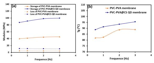
Fig. 9 (a and b): (a) The storage and loss modulus, and (b) the glass transition temperature as a function of frequency of PVC-PVA and PVC-PVA@CS QD membranes.
