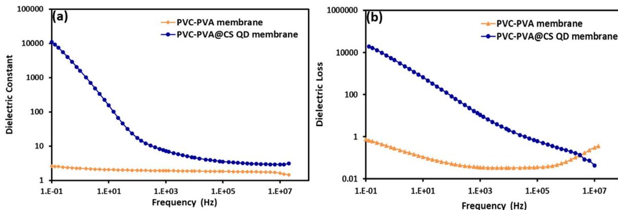
Fig. 12 (a and b): (a) The dielectric constant, and (b) dielectric loss as a function of frequency of PVC-PVA and PVC-PVA@CS QD membranes.
