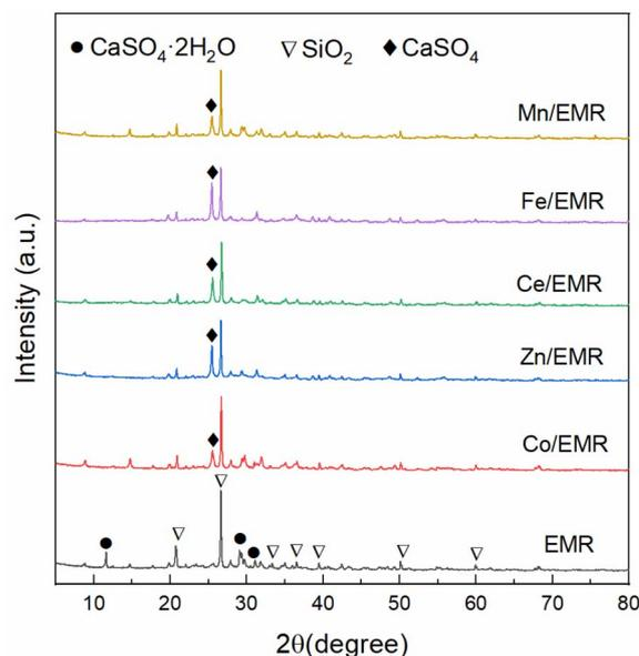
Fig. 1 XRD patterns of EMR and EMR-supported catalysts.
