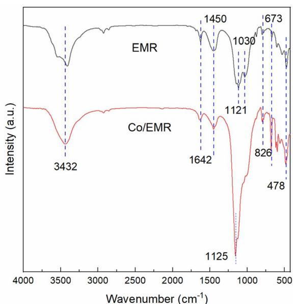
Fig. 2 FTIR spectra of EMR and Co/EMR.
