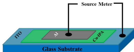
Scheme 1 Schematic representation of the fabricated metal–semiconductor (MS) junction device utilizing the Cu-IPA metallogel.
