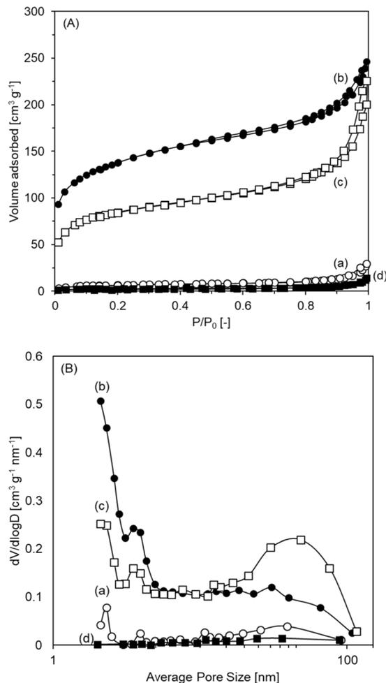
Fig. 4 (A) Nitrogen sorption isotherms and (B) pore-size distributions of ruthenium-encapsulated porous hollow silica spheres calcined at (a) 473, (b) 673, and (c) 873 K in air and (d) 673 K in an argon flow.
