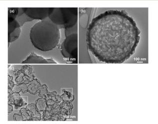
Fig. 1 TEM images of the ruthenium-encapsulated porous hollow silica sphere catalysts calcined at (a) 473, (b) 673, and (c) 873 K in air.
