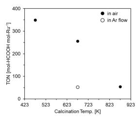
Fig. 5 Dependence of the activity for hydrogenation of carbon dioxide over ruthenium-encapsulated porous hollow silica sphere catalysts on calcination temperature.
