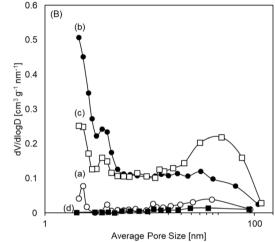
Fig. 4 (A) Nitrogen sorption isotherms and (B) pore-size distributions of ruthenium-encapsulated porous hollow silica spheres calcined at (a) 473, (b) 673, and (c) 873 K in air and (d) 673 K in an argon flow.
