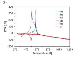
Fig. 2 (A) TG and (B) DTA curves of ruthenium-encapsulated porous hollow silica sphere catalysts calcined at (a) 473, (b) 673, (c) 873 K in air and (d) 673 K in an argon flow; (e) spherical carbon templates; and (f) pristine CTAB. Conditions: 20 K min $^{-1}$  in air.
