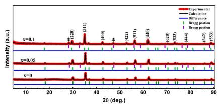
Fig. 2 Rietveld refined XRD pattern of the spinel  $ZnCe_xFe_{2-x}O_4$  nanofibers (x = 0, 0.05, 0.1).
