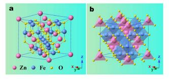
Fig. 1 The crystal structure and chemical composition of normal spinel ZFO and ZCFO ferries. (a) Ball-and-stick mode of normal spinel ZFO unit cell. The pink and blue spheres represent Zn cations and Fe cations, respectively, and O anions are in yellow. (b) Polyhedral model. Zn cations are located in tetrahedral A sites marked in pink. Fe cations are located in octahedral B sites marked in blue.
