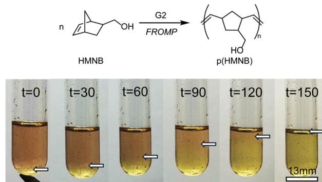
Fig. 1 5-Hydroxymethyl-2-norbornene (HMNB) Frontal Ring Opening Metathesis Polymerization (FROMP) with M/I = 10 000 HMNB (2.0 g, 16 mmol) and G2 (1.4 mg, 1.6  $\mu\text{mol}$ ). The bottom of the tube was touched directly with a soldering iron to initiate the reaction. Arrows denote the propagation front. The reported time is in seconds. Saturation and contrast were changed evenly for each time stamp.
