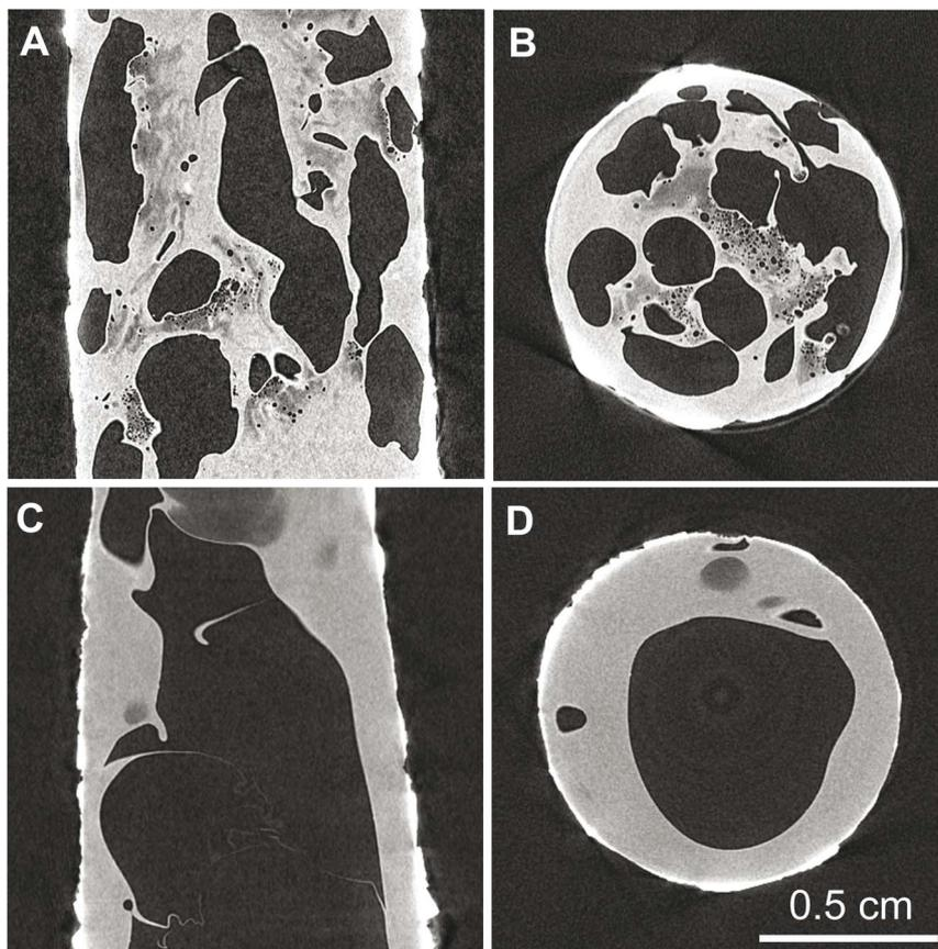
Fig. 3 Microcomputed tomography images of the HMNB foam prepared with *n*-pentane as the blowing agent. (A) Frontal cross section of the 10 wt% foam (B) superior cross section of the 10 wt% foam (C) frontal cross section of the 20 wt% foam (D) superior cross section of the 20 wt% foam.
