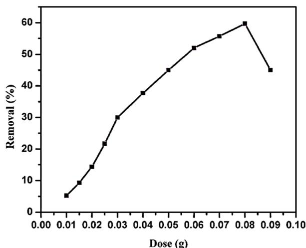
Fig. 7 Effect of the GR doses on the 150 mg L<sup>-1</sup> of MO adsorption at 25 °C and pH 7.0 in 25 mL solution.
