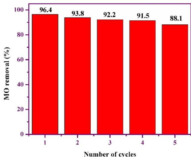
Fig. 10 Regeneration of GR adsorbent towards MO.
