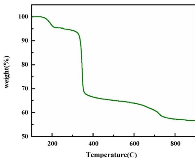
Fig. 5 The TGA curve of the GR.
