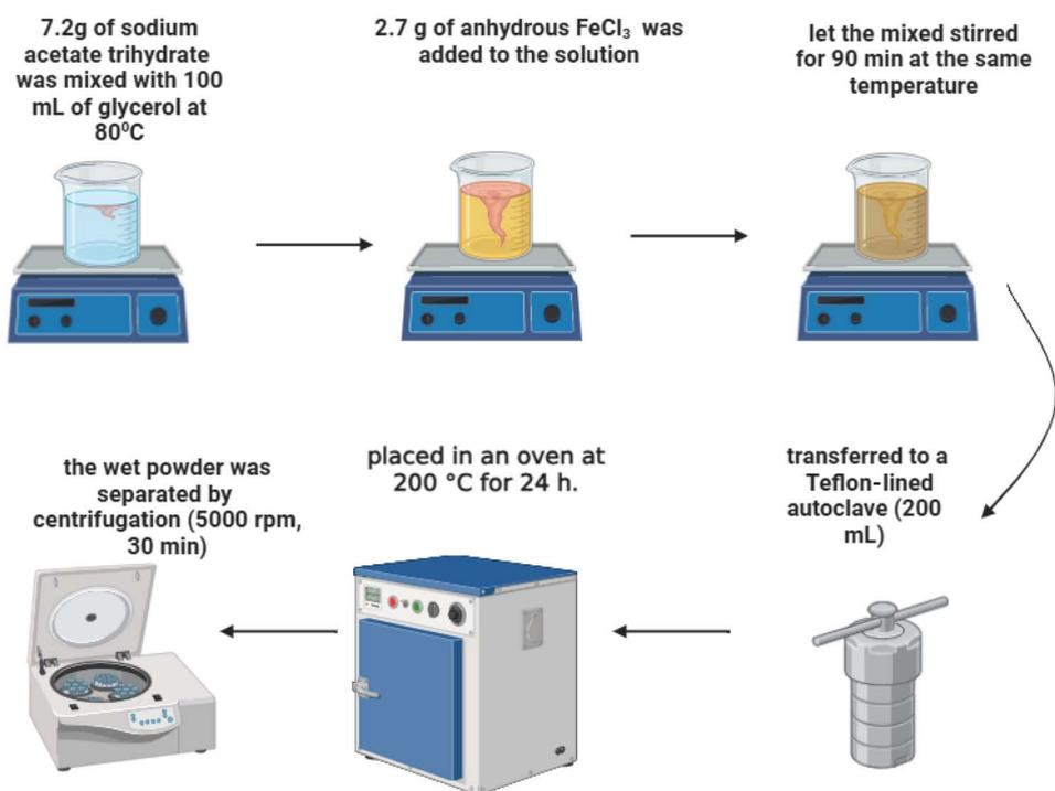
Fig. 1 Schematic representation of the GR preparation process.
