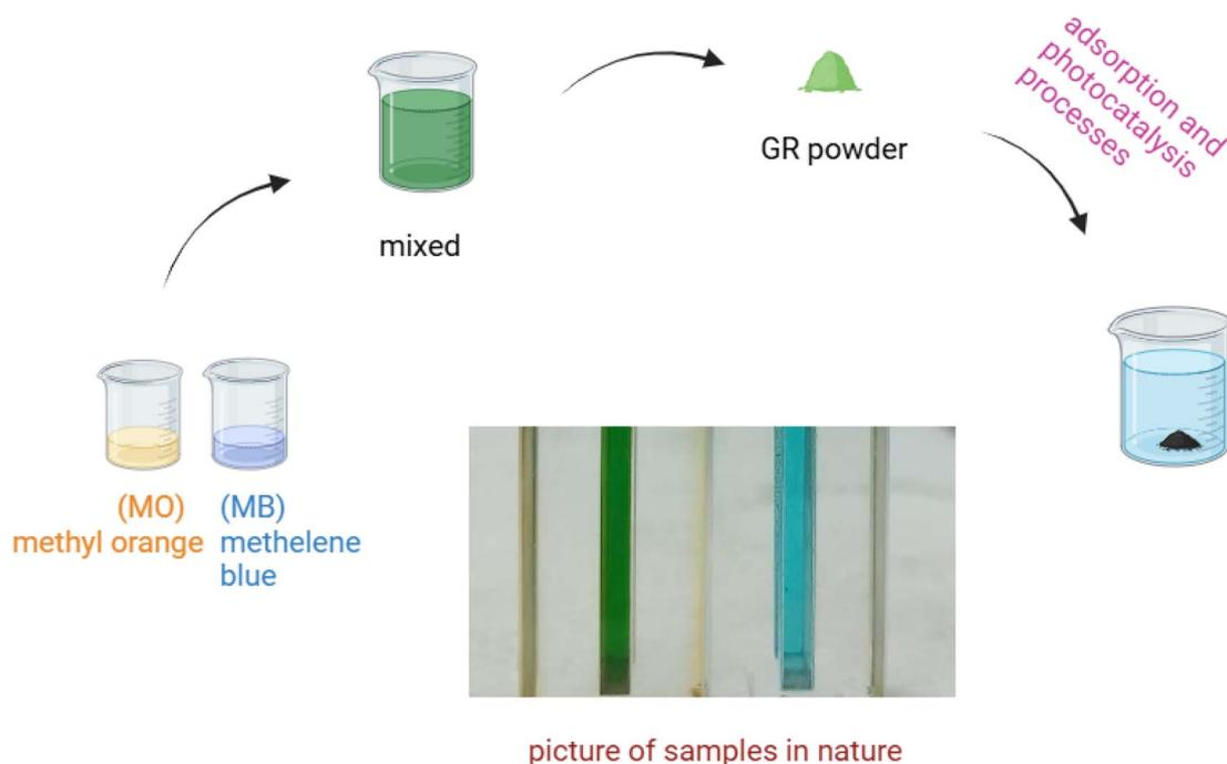
Fig. 17 Removing mixed of anionic dye (MO 12.5 mL at 30 mg L<sup>-1</sup>) and cationic dye (MB, 12.5 mL at 30 mg L<sup>-1</sup>) at pH 7.0 and 25 °C.
