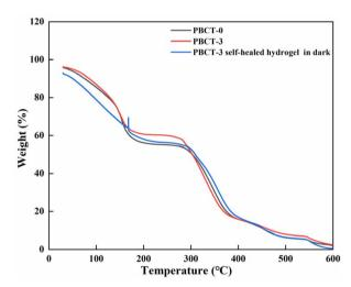
Fig. 5 TG curves of the self-healed PBCT hydrogel.
