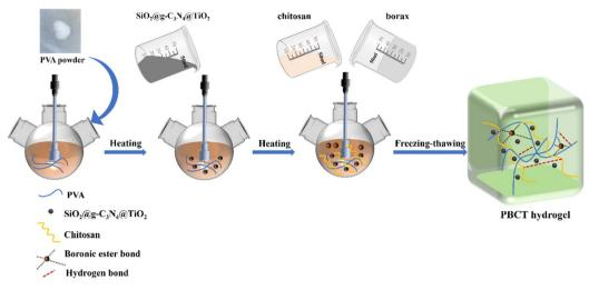
Fig. 1 Preparation route of the PBCT hydrogel.
