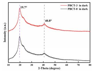
Fig. 4 XRD patterns of PBCT-0 and PBCT-3 hydrogels.
