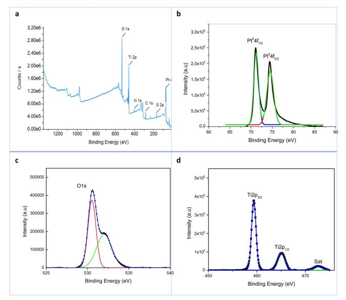
Fig. 2 XPS spectra of Pt-NPs/TiO<sub>2</sub>-NTs prepared by electrodeposition under potential of about 0.1 V.
