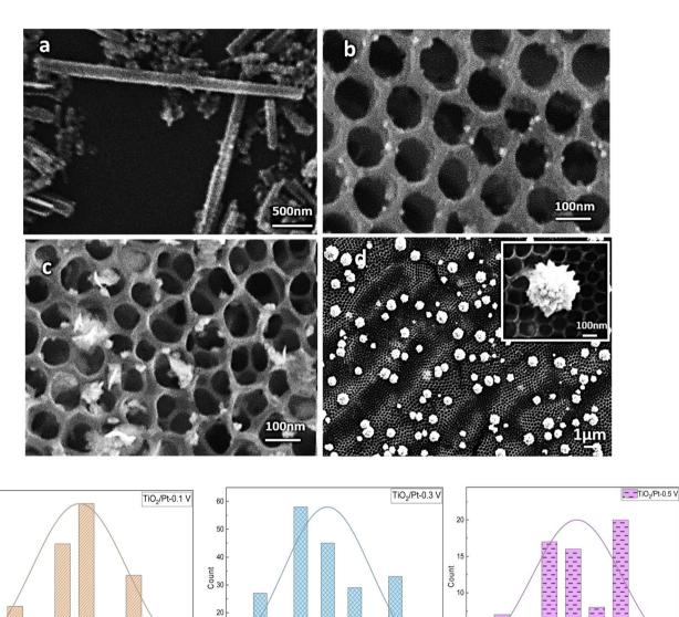
Fig. 3 The SEM images and nanoparticle size distribution of (a)  $TiO_2$ -NTs and  $Pt/TiO_2$ -NTs deposited in different voltages (b) 0.1 V, (c) 0.3 V and (d) 0.5 V.
