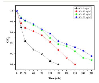
Fig. 8 Ethyl acetate degradation as a function of time for different initial concentrations using  $Pt/TiO_2$  catalyst prepared at 0.1 V.
