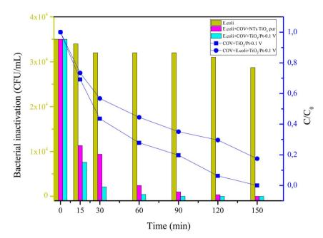
Simultaneous removal of E. coli and ethyl acetate as a function of irradiation time for pure TiO2 nanotubes and Pt/TiO2-NTs.
