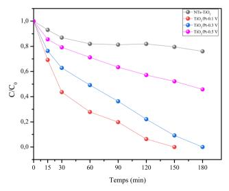
Fig. 7 Photocatalytic degradation of ethyl acetate as a function of time of pure and Pt-NPs decorated TiO<sub>2</sub>-NTs prepared by electrodeposition at different potentials.
