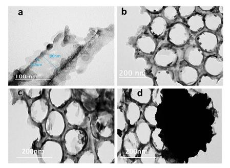
Fig. 4 TEM micrographs of the investigated Pt/TiO<sub>2</sub>-NTs catalysts (a) prepared at different potential (b) 0.1 V, (c) 0.3 V and (d) 0.5 V.
