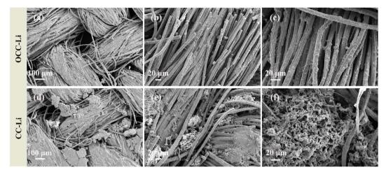
Fig. 8 Electrode morphology of symmetrical cells after 50 cycles at 1 mA cm<sup>-2</sup>, 1 mA h cm<sup>-2</sup> (a-c) OCC-Li and (d-f) CC-Li.
