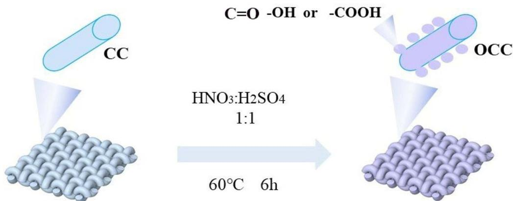
Fig. 1 Schematic diagram of the OCC preparation process.
