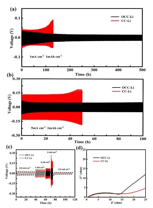
Fig. 7 The OCC-Li $\parallel$ OCC-Li and CC-Li $\parallel$ CC-Li symmetrical cells for 1 mA h cm $^{-2}$  (a and b) voltage curves at 1 mA cm $^{-2}$  and 5 mA cm $^{-2}$ ; (c) rate performance; (d) EIS Nyquist plots.
