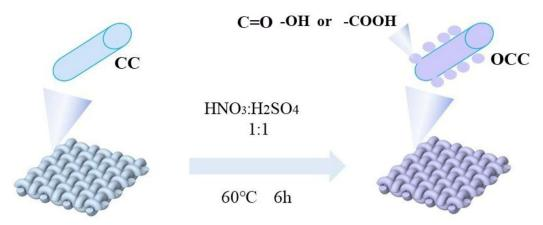
Fig. 1 Schematic diagram of the OCC preparation process.
