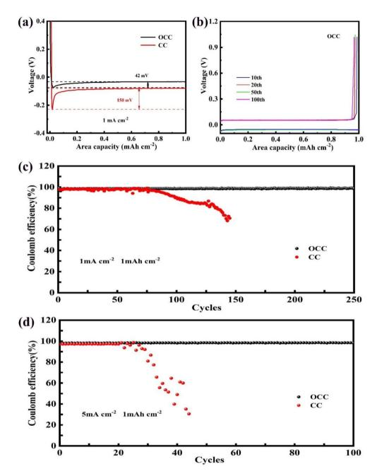
Fig. 6 (a) Nucleation overpotentials of Li on the OCC and CC at  $1 \, \text{mA cm}^{-2}$ . (b) Voltage-capacity curves of the OCC||Li at different cycles. (c and d) CE of the OCC||Li and CC||Li cells at  $1 \, \text{mA cm}^{-2}$  and  $5 \, \text{mA cm}^{-2}$ .
