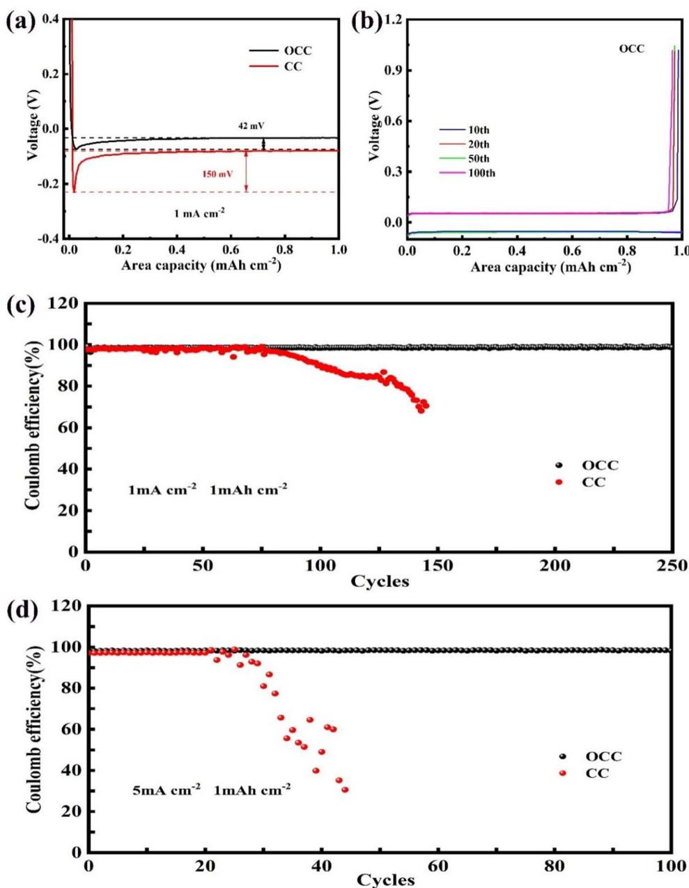
Fig. 6 (a) Nucleation overpotentials of Li on the OCC and CC at 1 mA cm<sup>-2</sup>. (b) Voltage–capacity curves of the OCC||Li at different cycles. (c and d) CE of the OCC||Li and CC||Li cells at 1 mA cm<sup>-2</sup> and 5 mA cm<sup>-2</sup>.
