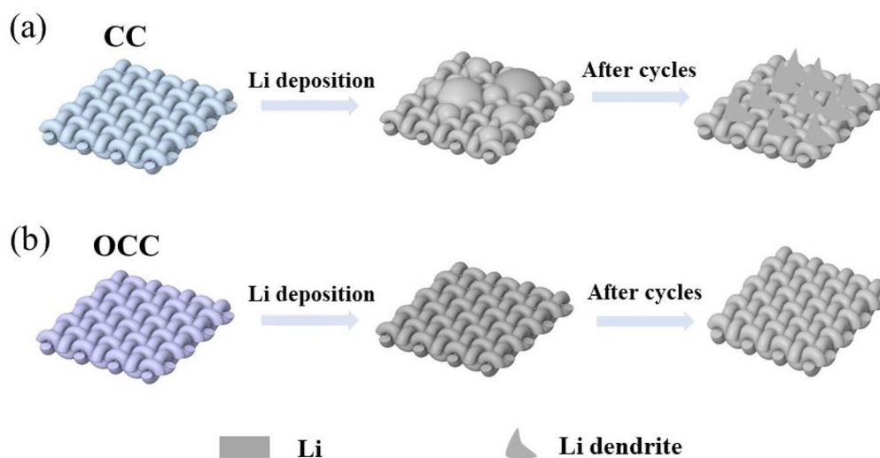
Fig. 2 The diagram of Li deposition on the (a) CC and (b) OCC.
