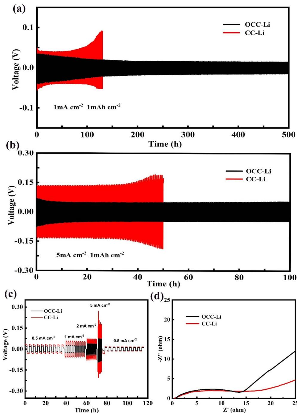
Fig. 7 The OCC-Li||OCC-Li and CC-Li||CC-Li symmetrical cells for 1 mA h cm<sup>-2</sup> (a and b) voltage curves at 1 mA cm<sup>-2</sup> and 5 mA cm<sup>-2</sup>; (c) rate performance; (d) EIS Nyquist plots.
