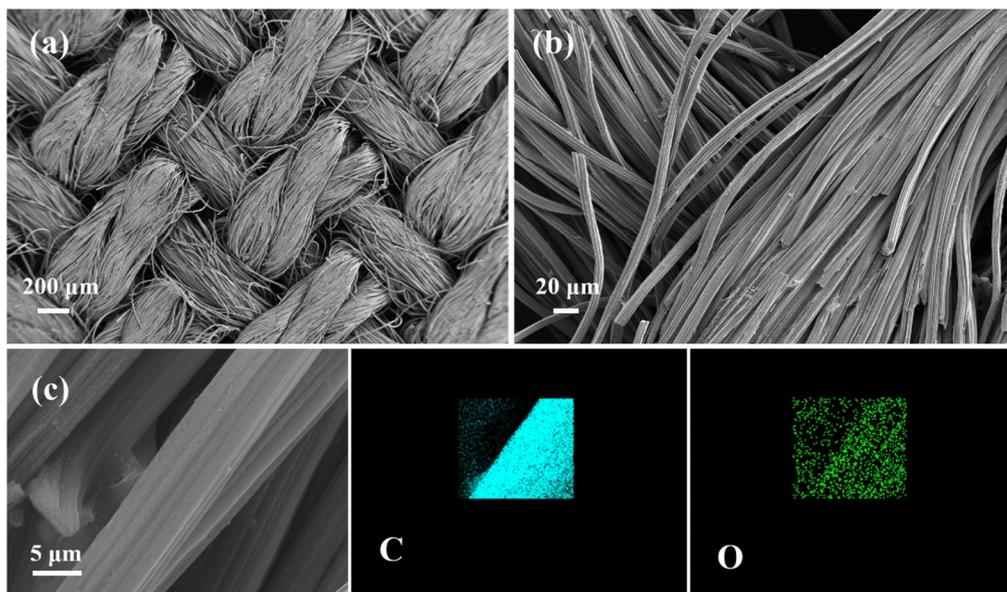
Fig. 3 (a and b) SEM images of the OCC. (c) EDS mapping images of the OCC.
