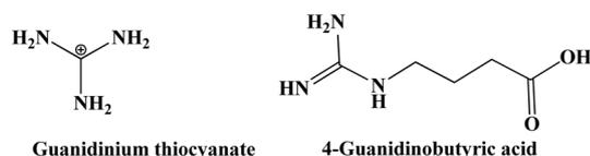
Fig. 17 Chemical structure of guanidinium cation and 4-guanidinobutyric acid additives.
