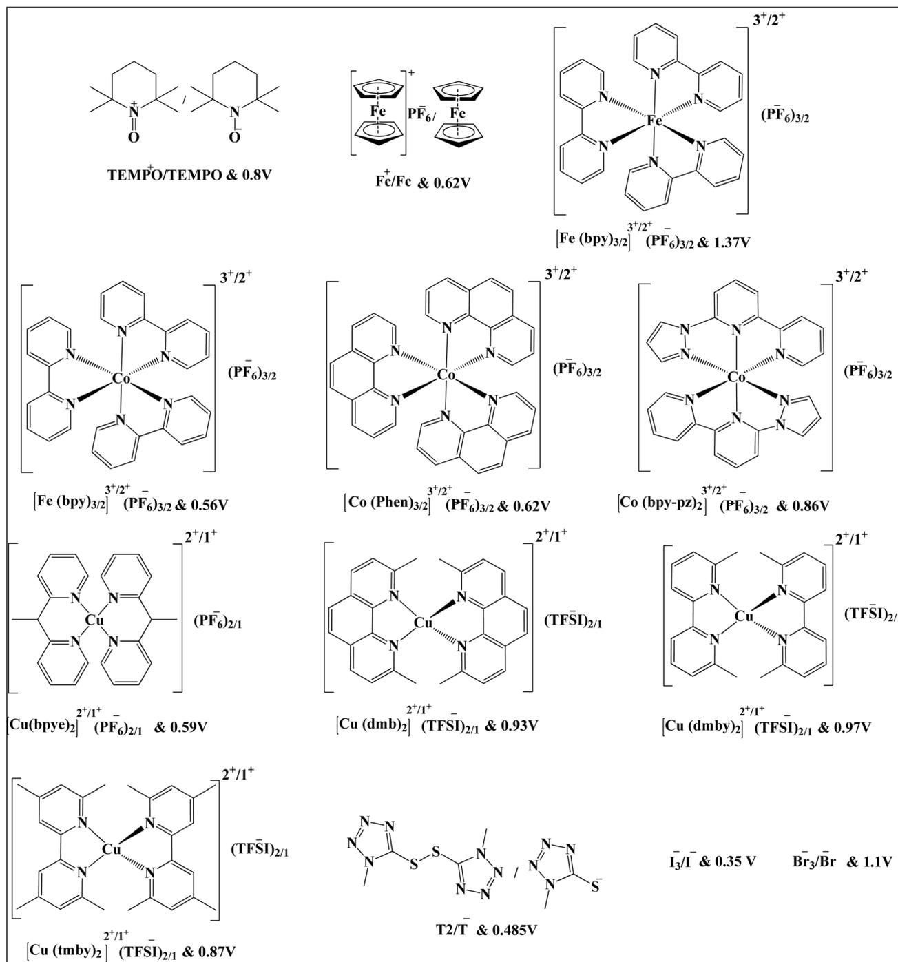
Fig. 13 Chemical structures of the most common redox couples used in DSSCs along with their standard redox potential. Where: TEMPO is 2,2,6,6-tetramethyl-1-piperidinyloxy & T<sub>2</sub> (dimer of 5-mercapto-1-methyltetrazole ion) & T<sup>-</sup> (5-mercapto-1-methyltetrazole ion).
