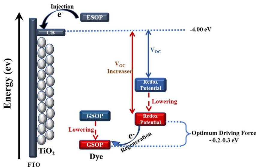
Fig. 12 Shows a strategy for boosting the  $V_{OC}$  by concurrently moving the redox couple potential and the dye's ground-state oxidation potential (GSOP) to higher positive values, resulting in an ideal driving force for rapid dye regeneration.
