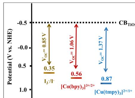
Fig. 14 Redox potential values and the corresponding  $V_{OC}$  values of the most common and efficient redox couples used in DSSCs, including  $I_3^-/I^-$ ,  $[Co(bpy)_3]^{3+}/^{2+}$ , and  $[Cu(tmpy)_3]^{2+}/^{1+}$ .
