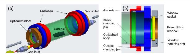
Fig. 1 (a) Framework of the versatile optical cell, and (b) expanded view of the window assembly.
