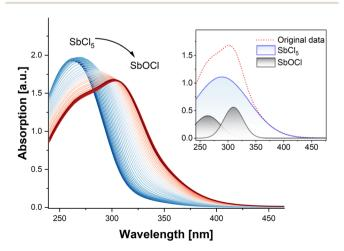
Fig. 7 UV-vis spectra of SbCl $_{\rm 5}$  vapor species, decomposed to SbCl $_{\rm 3}$  at 350 °C.
