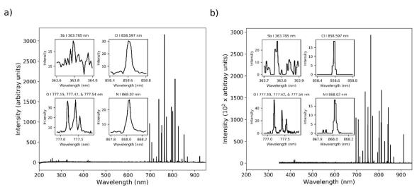
Fig. 8 LIBS spectra of SbCl $_5$  vapor in Ar gas. (a) Data from the 200–1000 nm spectrometer, taken at 28 mJ with a gate delay of 3  $\mu$ s and is an accumulation of 20 shots, and (b) data from the 350–950 nm spectrometer taken at 26 mJ and 2  $\mu$ s gate delay and is an accumulation of 120 shots.
