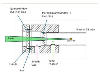
Fig. 6 Schematic of the double-window optical cell design.
