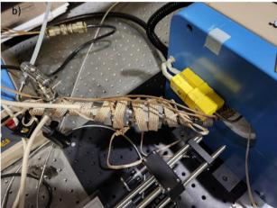
Fig. 2 (a) Picture of the external sampling chamber without the heat tape and (b) a photo of the external sample chamber with added heat tape before wrapping with silicone insulation tape.
