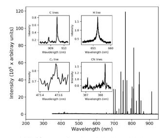
Fig. 5 A full LIBS spectrum from the optical cell in naphthalene vapor at 85 °C, including CN, H,  $C_2$ , and C lines at 2 us gate delay and 43 mJ. The spectrum is an accumulation of 740 shots.
