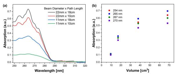
Fig. 3 (a) Average spectra of naphthalene vapor at steady-state at 85 °C. Beam diameter and path length were varied to determine optimal configuration. The strongest signal was observed at a 22 mm beam diameter and 18 cm path length. (b) Scatter plot of beam interaction volume and peak intensities at select wavelengths.
