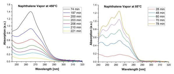
Fig. 4 (Left) Average curves for naphthalene vapor at 450 °C over time, showing sample depletion at the end of the test. (Right) Average curves for naphthalene vapor at 85 °C over time, showing the increase of naphthalene concentration at the start of the test.
