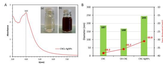
Fig. 1 (A) Electronic absorption spectra of a CNCs-AgNPs suspension in water. Inset images: photographs of ox-CNCs (a) and CNCs-AgNPs (b) suspensions; (B) average particle size and zeta potential of CNCs, ox-CNCs, and CNCs-AqNPs.
