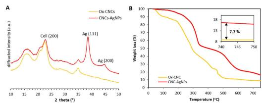
Fig. 3 (A) XRD profiles of ox-CNCs (orange) and CNCs-AqNPs (red); (B) TGA thermograms for ox-CNCs (orange), and CNCs-AqNPs (red).
