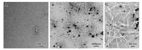
Fig. 2 TEM images of negatively stained preparations form suspensions of initial CNCs (A) and CNCs-AgNPs (B and C). The AgNPs appear as black dots.
