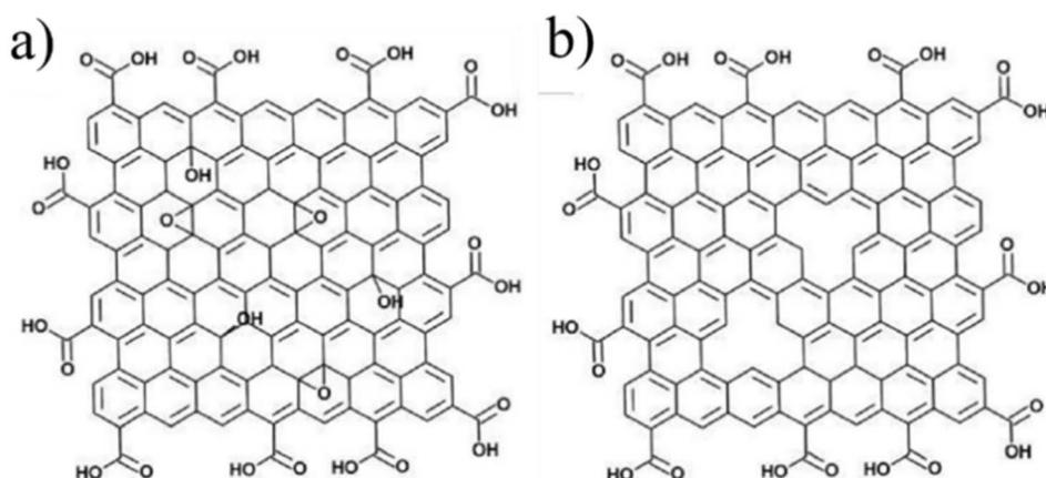
Fig. 8 Chemical structure models of (a) graphene oxide (GnO) and (b) reduced graphene oxide (rGnO).<sup>11</sup> Reproduced from ref. 11 with permission from De Gruyter as part of a partnership with IUPAC, copyright 2011.
