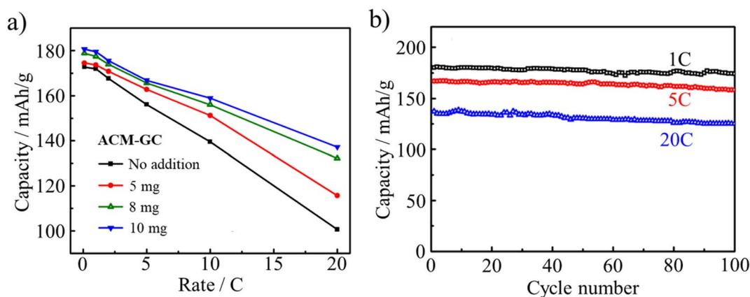
Fig. 30 LIB performances of  $\text{Li}_4\text{Ti}_5\text{O}_{12}$  (LTO) anode coated with ACM-GC: (a) rate performances as a function of ACM-GC dosage and (b) cycle performances of LTO coated with ACM-GC at  $10 \text{ mg}_{\text{ACM}}/\text{g}_{\text{LTO}}$  dosage at different rates.<sup>87</sup> Reproduced from ref. 87 with permission from Elsevier Ltd, copyright 2012.
