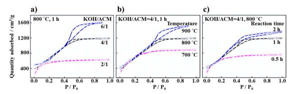
Fig. 21  $N_2$  adsorption/desorption isotherms at 77 K for mesoporous carbons prepared from ACM-GC: effects of (a) KOH/ACM ratio, (b) heat treatment temperature and (c) heating time. Reproduced from ref. 8 with permission from Elsevier Ltd, copyright 2011.
