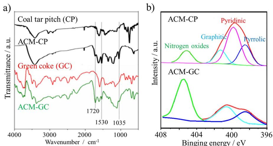
Fig. 3 ACMs derived from coal tar pitch (CP) and green coke (GC): (a) FTIR and (b) N 1s XPS spectra.<sup>7,9</sup> Reproduced from ref. 7 with permission from the Royal Society of Chemistry, copyright 2013. Reproduced from ref. 9 with permission from Science Press, copyright 2015.
