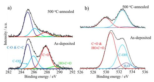
Fig. 12 XPS spectra for GnO films prepared using Hummers' method after deposition on  $Si_3N_4/SiO_2$  substrate and after heat-treatment at 500 °C: (a) C 1s and (b) O 1s spectra. <sup>38</sup> Reproduced from ref. 38 with permission from Elsevier Ltd, copyright 2010.
