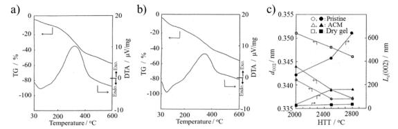
Fig. 7 ACMs prepared from raw coke: TG and DTA curves (10 °C min<sup>-1</sup>) for (a) ACM and (b) its dry gel prepared in NH<sub>3</sub>·H<sub>2</sub>O, and (c) changes in  $d_{002}$  interlayer spacing and  $L_c$ (002) crystallite size with heat treatment temperature for the pristine raw coke, ACM and its dry gel.<sup>14</sup> Reproduced from ref. 14 with permission from the Carbon Society of Japan, copyright 1993.
