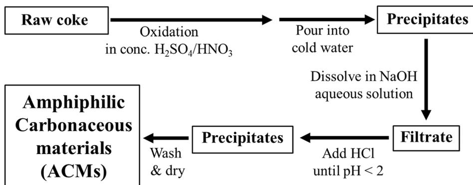
Fig. 2 Flow diagram for the preparation of ACMs.
