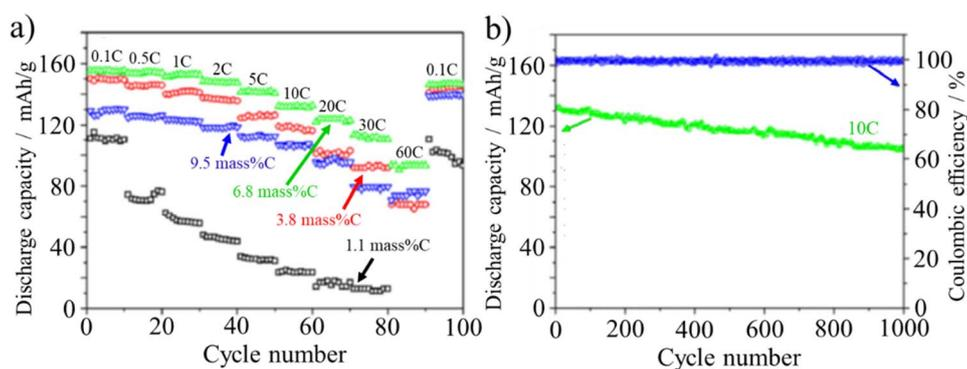
Fig. 31 Cyclic performances of LIBs with carbon-coated  $\text{LiFePO}_4$  cathode by ACM-CP: (a) discharge capacities at different current densities from 0.1C to 60C and (b) discharge capacity and coulombic efficiency vs. cycle numbers up to 1000 cycles at 10C rate.<sup>88</sup> Reproduced from ref. 88 with permission from Elsevier Ltd, copyright 2014.
