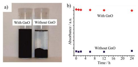
Fig. 36 Few-layered graphene oxide (GnO) helps dispersion of multi-walled carbon nanotubes in deionized water: (a) immediately after sonication and (b) absorbance of the two suspensions in (a) vs. standing still time.<sup>37</sup> Reproduced from ref. 37 with permission from the American Chemical Society, copyright 2010.
