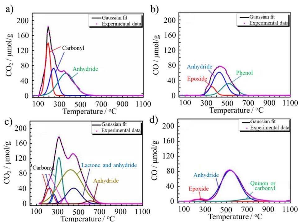
Fig. 4 TPD profiles of (a and b) ACM-CP<sup>25</sup> and (c and d) ACM-GC. Reproduced from ref. 25 with permission from Elsevier Ltd, copyright 2016.
