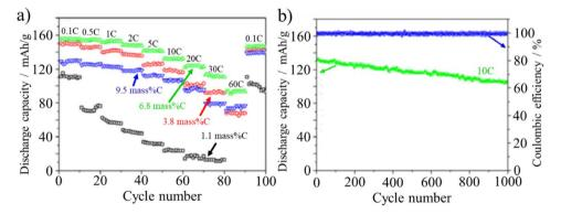
Fig. 31 Cyclic performances of LIBs with carbon-coated LiFePO<sub>4</sub> cathode by ACM-CP: (a) discharge capacities at different current densities from 0.1C to 60C and (b) discharge capacity and coulombic efficiency vs. cycle numbers up to 1000 cycles at 10C rate. Reproduced from ref. 88 with permission from Elsevier Ltd, copyright 2014.
