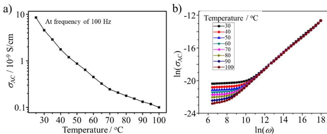
Fig. 10 AC conductivity ( $\sigma_{\text{AC}}$ ) of a  $\text{GnO}$  film: (a) temperature dependence at 100 Hz and (b) frequency,  $\omega$ , dependence at different temperatures.<sup>39</sup> Reproduced from ref. 39 with permission from Elsevier Ltd, copyright 2015.
