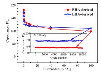
Fig. 24 Rate and cycle performances (inset) of LHA- and BHA-derived nanoporous carbons.<sup>17</sup> Reproduced from ref. 17 with permission from Elsevier Ltd, copyright 2014.
