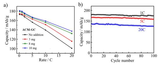
Fig. 30 LIB performances of  $\text{Li}_4\text{Ti}_5\text{O}_{12}$  (LTO) anode coated with ACM-GC: (a) rate performances as a function of ACM-GC dosage and (b) cycle performances of LTO coated with ACM-GC at 10 mg<sub>ACM</sub>/g<sub>LTO</sub> dosage at different rates.<sup>87</sup> Reproduced from ref. 87 with permission from Elsevier Ltd, copyright 2012.
