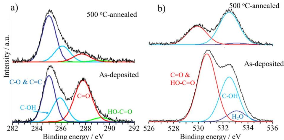
Fig. 12 XPS spectra for GnO films prepared using Hummers' method after deposition on  $\text{Si}_3\text{N}_4/\text{SiO}_2$  substrate and after heat-treatment at 500 °C: (a) C 1s and (b) O 1s spectra.<sup>38</sup> Reproduced from ref. 38 with permission from Elsevier Ltd, copyright 2010.
