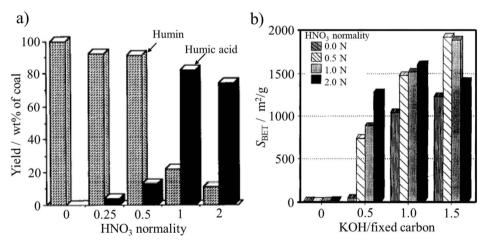
Fig. 26 Oxidation and activation of a bituminous coal: (a) yield of humin and humic acid as a function of HNO<sub>3</sub> normality and (b)  $S_{BET}$  of the resultant activated carbons as a function of KOH/coal ratio and HNO<sub>3</sub> normality used for oxidation.<sup>71</sup> Reproduced from ref. 71 with permission from Elsevier Ltd, copyright 1995.
