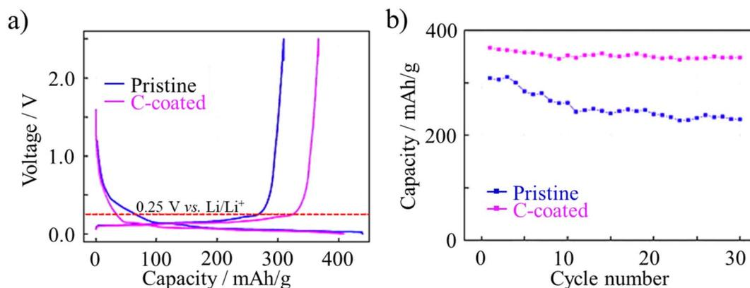
Fig. 28 LIBs using graphite anode with or without carbon-coating by ACM-GC: (a) charge/discharge curves and (b) cyclic performances at  $50 \text{ mA g}^{-1}$ .<sup>83</sup> Reproduced from ref. 83 with permission from Elsevier Ltd, copyright 2010.
