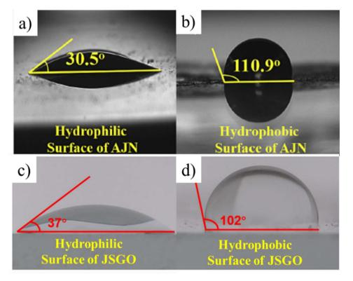
Fig. 15 Contact angles of water droplets on surfaces of AJN (a and b)<sup>44</sup> and JSGO (c and d).<sup>45</sup> (a and c) are on hydrophilic surfaces while (b and d) are on hydrophobic surfaces. Reproduced from ref. 44 with permission from Elsevier Ltd, copyright 2018; reproduced from ref. 45 with permission from Elsevier Ltd, copyright 2022.
