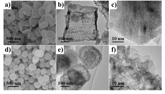
Fig. 34 SEM and TEM images of MnO<sub>2</sub> particles prepared from MnCO<sub>3</sub>/ACM mixture: (a-c) hollow cubes and (d-f) hollow spheres. (a and d) SEM images, and (b, c, e and f) TEM images. 102 Reproduced from ref. 102 with permission from the American Chemical Society, copyright 2014.
