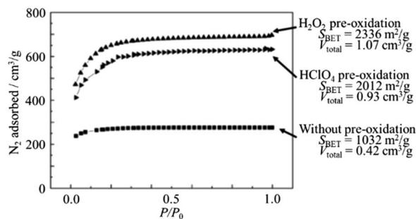
Fig. 27  $N_2$  adsorption isotherms of the activated carbons derived from petroleum coke with or without pre-oxidation.<sup>78</sup> Reproduced from ref. 78 with permission from Elsevier Ltd, copyright 2008.
