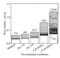
Fig. 25 Histogram of the different types of pores in carbons prepared from anthracite under various pre-oxidation conditions. The number shown for each column is total oxygen content ( $\mu$ mol g<sup>-1</sup>) after pre-oxidation.<sup>76</sup> Reproduced from ref. 76 with permission from Elsevier Ltd, copyright 1997.
