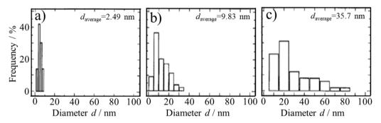
Fig. 32 Diameter distribution of Pt particles loaded on ACMs after heat treatment at different temperatures of (a) 500 °C, (b) 700 °C and (c) 1000 °C. 1000 Reproduced from ref. 100 with permission from Elsevier Ltd, copyright 1996.
