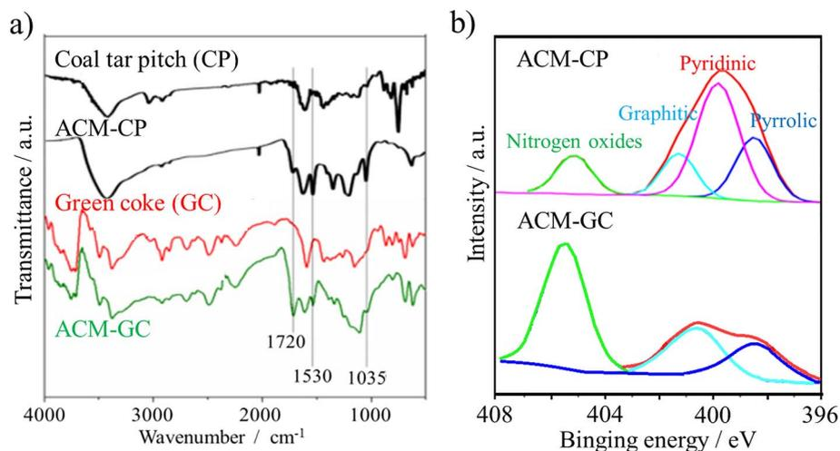
Fig. 3 ACMs derived from coal tar pitch (CP) and green coke (GC): (a) FTIR and (b) N 1s XPS spectra.<sup>7,9</sup> Reproduced from ref. 7 with permission from the Royal Society of Chemistry, copyright 2013. Reproduced from ref. 9 with permission from Science Press, copyright 2015.
