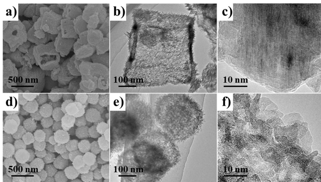
Fig. 34 SEM and TEM images of  $\text{MnO}_2$  particles prepared from  $\text{MnCO}_3/\text{ACM}$  mixture: (a–c) hollow cubes and (d–f) hollow spheres. (a and d) SEM images, and (b, c, e and f) TEM images.<sup>102</sup> Reproduced from ref. 102 with permission from the American Chemical Society, copyright 2014.
