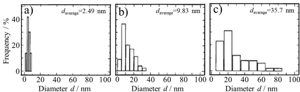
Fig. 32 Diameter distribution of Pt particles loaded on ACMs after heat treatment at different temperatures of (a) 500 °C, (b) 700 °C and (c) 1000 °C.<sup>100</sup> Reproduced from ref. 100 with permission from Elsevier Ltd, copyright 1996.
