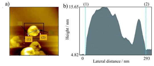
Fig. 1 (a) AFM image in tapping mode of ACM-CP on a mica flake and (b) height distribution of the particle in (a). Reproduced from ref. 7 with permission from the Royal Society of Chemistry, copyright 2013.
