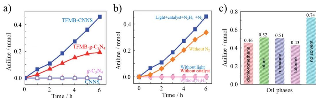
Fig. 38 Phase boundary photocatalysis of TEMB-CNNS for nitrobenzene reduction: production of aniline (a) in water phase, (b) under various conditions, and (c) for different oil phases.<sup>64</sup> Reproduced from ref. 64 with permission from the Royal Society of Chemistry, copyright 2019.
