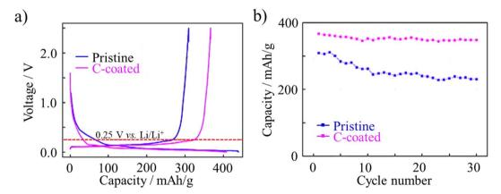
Fig. 28 LIBs using graphite anode with or without carbon-coating by ACM-GC: (a) charge/discharge curves and (b) cyclic performances at 50 mA  $g^{-1.83}$  Reproduced from ref. 83 with permission from Elsevier Ltd, copyright 2010.
