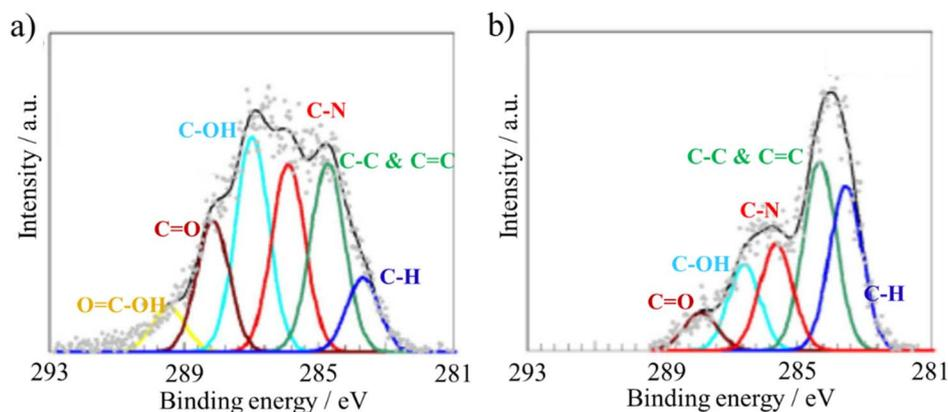
Fig. 13 XPS C 1s spectra of (a) as-prepared GnO film and (b) after 450 W microwave irradiation for 20 min.<sup>42</sup> Reproduced from ref. 42 with permission from Elsevier Ltd, copyright 2015.
