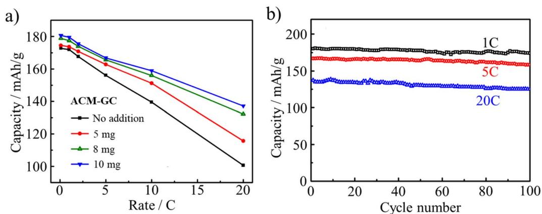
Fig. 30 LIB performances of  $\text{Li}_4\text{Ti}_5\text{O}_{12}$  (LTO) anode coated with ACM-GC: (a) rate performances as a function of ACM-GC dosage and (b) cycle performances of LTO coated with ACM-GC at  $10 \text{ mg}_{\text{ACM}}/\text{g}_{\text{LTO}}$  dosage at different rates.<sup>87</sup> Reproduced from ref. 87 with permission from Elsevier Ltd, copyright 2012.
