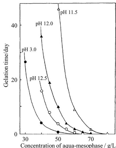
Fig. 6 Effects of concentration of ACM and pH on the gelation time of a mesophase-pitch-derived ACM in an  $\text{NH}_3 \cdot \text{H}_2\text{O}$  aqueous solution at 25 °C.<sup>12</sup> Reproduced from ref. 12 with permission from Elsevier Ltd, copyright 1991.
