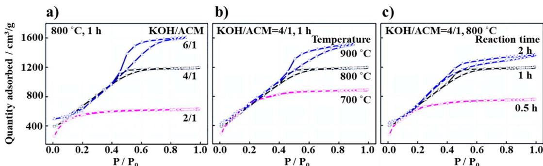
Fig. 21 N<sub>2</sub> adsorption/desorption isotherms at 77 K for mesoporous carbons prepared from ACM-GC: effects of (a) KOH/ACM ratio, (b) heat treatment temperature and (c) heating time.<sup>8</sup> Reproduced from ref. 8 with permission from Elsevier Ltd, copyright 2011.
