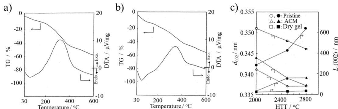
Fig. 7 ACMs prepared from raw coke: TG and DTA curves ( $10\text{ }^{\circ}\text{C min}^{-1}$ ) for (a) ACM and (b) its dry gel prepared in  $\text{NH}_3 \cdot \text{H}_2\text{O}$ , and (c) changes in  $d_{002}$  interlayer spacing and  $L_c(002)$  crystallite size with heat treatment temperature for the pristine raw coke, ACM and its dry gel.<sup>14</sup> Reproduced from ref. 14 with permission from the Carbon Society of Japan, copyright 1993.
