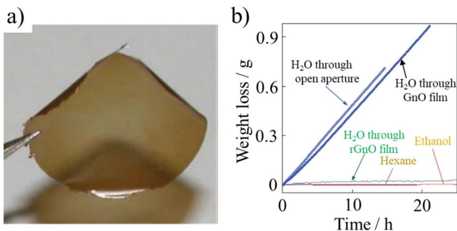
Fig. 39 Water-permeable ZnO films: (a) digital photograph of the film and (b) weight loss of water for a container sealed with a ZnO film (film thickness  $\approx 1 \mu\text{m}$ ; aperture area  $\approx 1 \text{cm}^2$ ). No loss was detected for ethanol, and hexane, but water was evaporated from the container as freely as through an open aperture.<sup>125</sup> Reproduced from ref. 125 with permission from the American Association for the Advancement of Science, copyright 2012.
