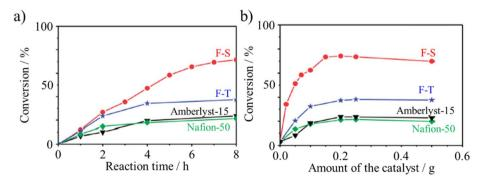
Fig. 33 Conversion of pivalic acid over sulfonated carbon catalysts (F–S and F–T) in comparison with two commercially available catalysts (Amberlyst-15 and Nafion-15) at 70 °C: (a) conversion kinetics using various catalysts (catalyst: 0.5 g, pivalic acid: 1.02 g and methanol: 1.60 g) and (b) effect of catalyst amount (pivalic acid: 1.02 g and methanol:1.60 g).<sup>62</sup> Reproduced from ref. 62 with permission from the Royal Society of Chemistry, copyright 2014.
