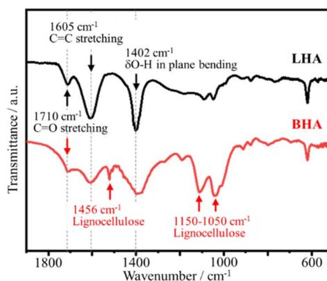
Fig. 17 FTIR spectra of biotechnology humic acid (BHA) and leonardite humic acid (LHA).<sup>17</sup> Reproduced from ref. 17 with permission from Elsevier Ltd, copyright 2014.
