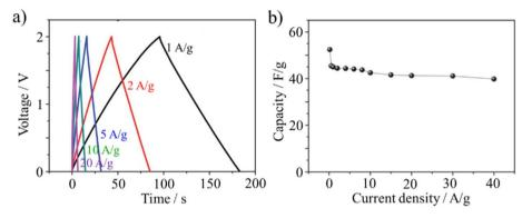
Fig. 23 Asymmetric capacitor of MnO<sub>2</sub>|1 M Na<sub>2</sub>SO<sub>4</sub> aqueous electrolyte|ACM-CP-derived carbon: (a) charge/discharge curves at different current densities and (b) rate performance.7 Reproduced from ref. 7 with permission from the Royal Society of Chemistry, copyright 2013.
