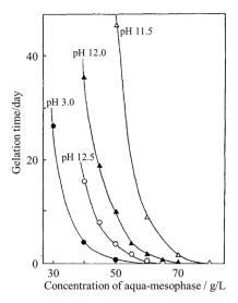
Fig. 6 Effects of concentration of ACM and pH on the gelation time of a mesophase-pitch-derived ACM in an NH<sub>3</sub>·H<sub>2</sub>O aqueous solution at 25 °C.12 Reproduced from ref. 12 with permission from Elsevier Ltd, copyright 1991.
