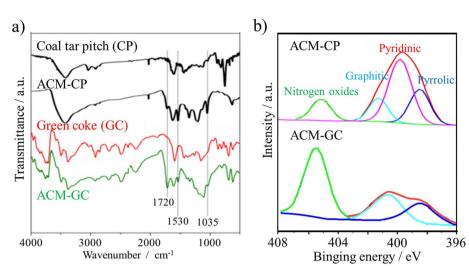
Fig. 3 ACMs derived from coal tar pitch (CP) and green coke (GC): (a) FTIR and (b) N 1s XPS spectra.<sup>7,9</sup> Reproduced from ref. 7 with permission from the Royal Society of Chemistry, copyright 2013. Reproduced from ref. 9 with permission from Science Press, copyright 2015.
