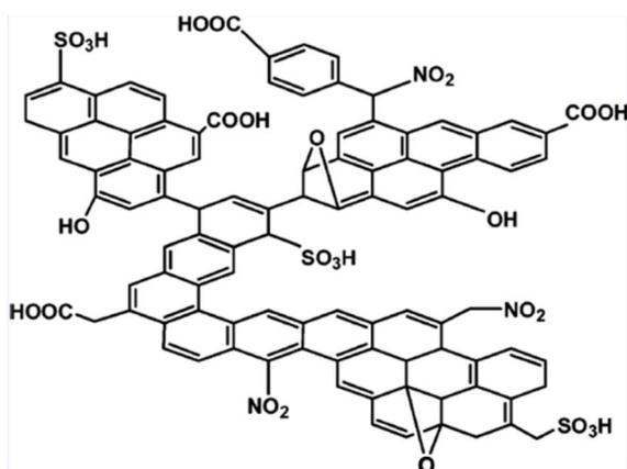
Fig. 5 Structural model for ACM-CP.<sup>21</sup> Reproduced from ref. 21 with permission from the American Chemical Society, copyright 2014.
