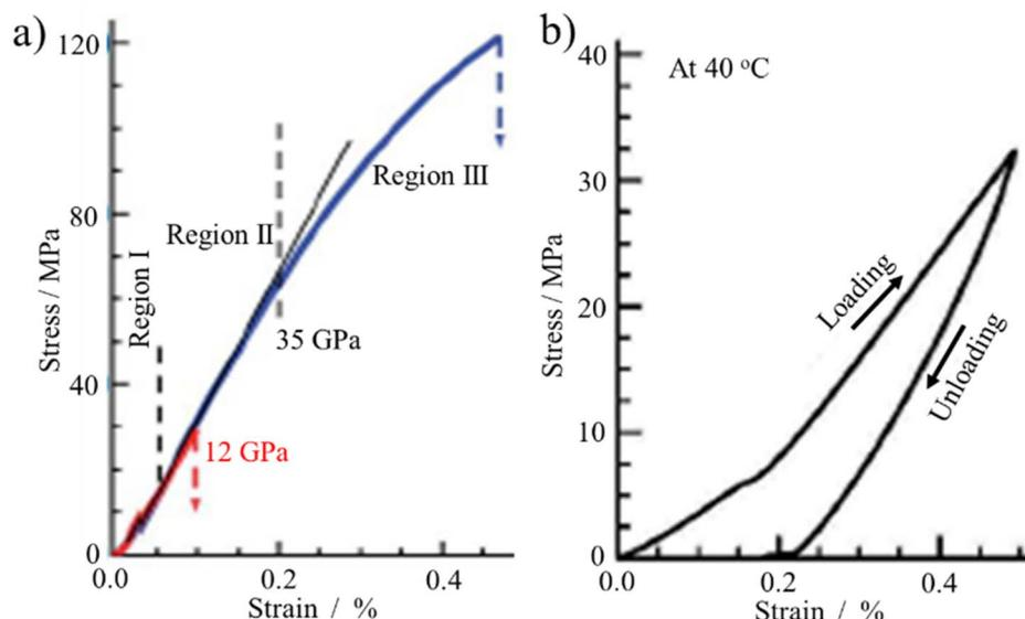
Fig. 11 Stress–strain behavior of  $\text{GnO}$  films under tension: (a) stress–strain curve and (b) loading–unloading in region I in (a).<sup>41</sup> Reproduced from ref. 41 with permission from Springer Nature Publishing Group, copyright 2007.
