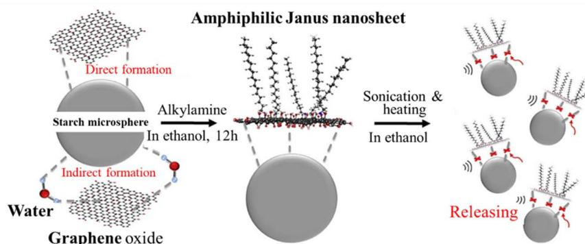
Fig. 14 Illustration of the synthesis of graphene-based AJNs using temporary substrates of starch microspheres.<sup>44</sup> Reproduced from ref. 44 with permission from Elsevier Ltd, copyright 2018.
