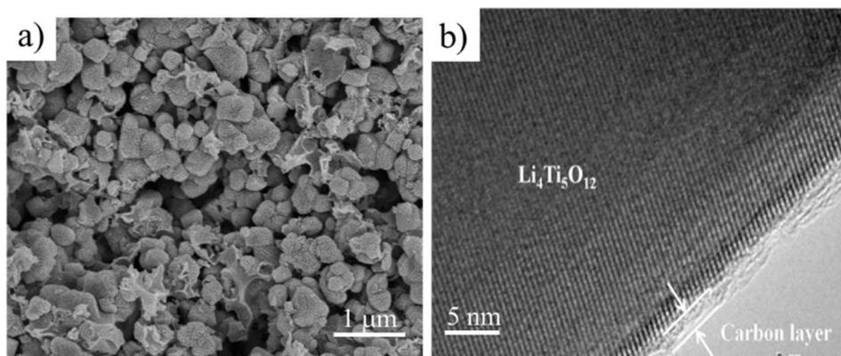
Fig. 29 (a) SEM image and (b) TEM image of carbon-coated  $\text{Li}_4\text{Ti}_5\text{O}_{12}$  using ACM-GC.<sup>87</sup> Reproduced from ref. 87 with permission from Elsevier Ltd, copyright 2012.
