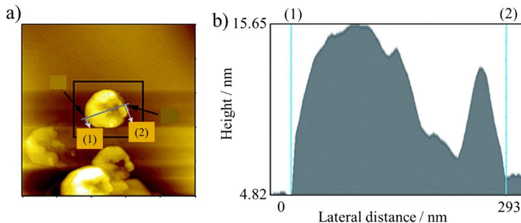
Fig. 1 (a) AFM image in tapping mode of ACM-CP on a mica flake and (b) height distribution of the particle in (a).<sup>7</sup> Reproduced from ref. 7 with permission from the Royal Society of Chemistry, copyright 2013.
