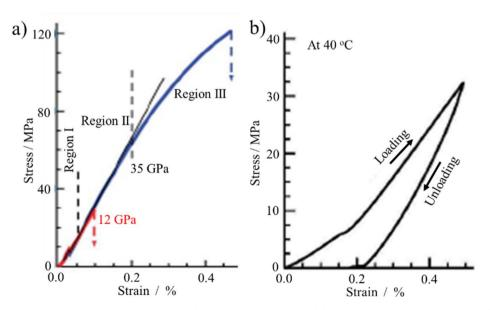
Fig. 11 Stress-strain behavior of GnO films under tension: (a) stress-strain curve and (b) loading-unloading in region I in (a).<sup>41</sup> Reproduced from ref. 41 with permission from Springer Nature Publishing Group, copyright 2007.
