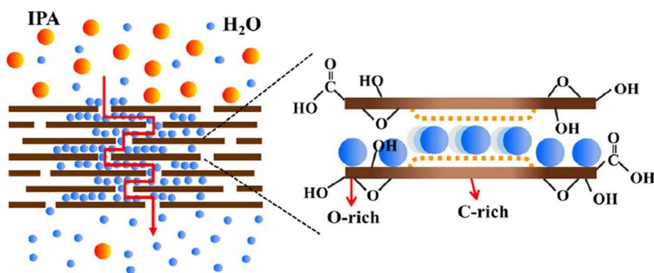
Fig. 37 Schematic of the mechanism for separating H<sub>2</sub>O from isopropanol using a pressure-assisted self-assembled few-layered GnO film.<sup>40</sup> Reproduced from ref. 40 with permission from Elsevier Ltd, copyright 2014.
