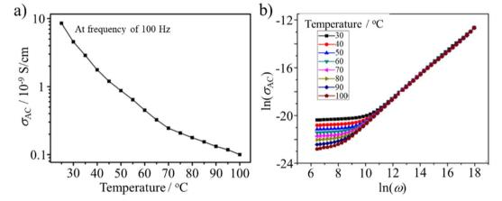
Fig. 10 AC conductivity ( $\sigma_{AC}$ ) of a GnO film: (a) temperature dependence at 100 Hz and (b) frequency,  $\omega$ , dependence at different temperatures.<sup>39</sup> Reproduced from ref. 39 with permission from Elsevier Ltd, copyright 2015.
