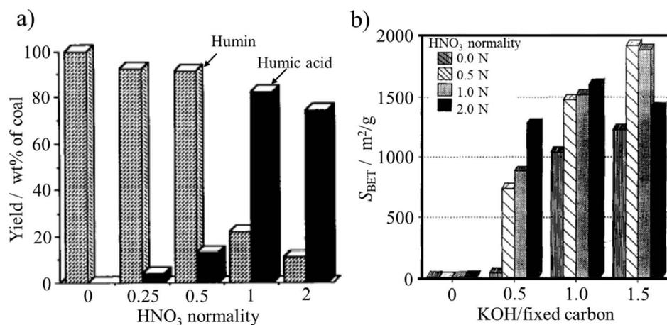
Fig. 26 Oxidation and activation of a bituminous coal: (a) yield of humin and humic acid as a function of  $\text{HNO}_3$  normality and (b)  $S_{\text{BET}}$  of the resultant activated carbons as a function of  $\text{KOH}/\text{coal}$  ratio and  $\text{HNO}_3$  normality used for oxidation.<sup>71</sup> Reproduced from ref. 71 with permission from Elsevier Ltd, copyright 1995.
