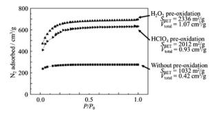
Fig. 27  $N_2$  adsorption isotherms of the activated carbons derived from petroleum coke with or without pre-oxidation. Reproduced from ref. 78 with permission from Elsevier Ltd, copyright 2008.
