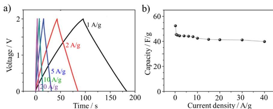
Fig. 23 Asymmetric capacitor of  $\text{MnO}_2|1 \text{ M Na}_2\text{SO}_4$  aqueous electrolyte|ACM-CP-derived carbon: (a) charge/discharge curves at different current densities and (b) rate performance.<sup>7</sup> Reproduced from ref. 7 with permission from the Royal Society of Chemistry, copyright 2013.
