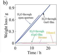
Fig. 39 Water-permeable GnO films: (a) digital photograph of the film and (b) weight loss of water for a container sealed with a GnO film (film thickness  $\approx 1 \, \mu m$ ; aperture area  $\approx 1 \, cm^2$ ). No loss was detected for ethanol, and hexane, but water was evaporated from the container as freely as through an open aperture. Reproduced from ref. 125 with permission from the American Association for the Advancement of Science, copyright 2012.
