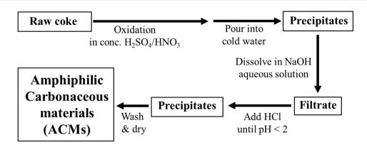
Fig. 2 Flow diagram for the preparation of ACMs.
