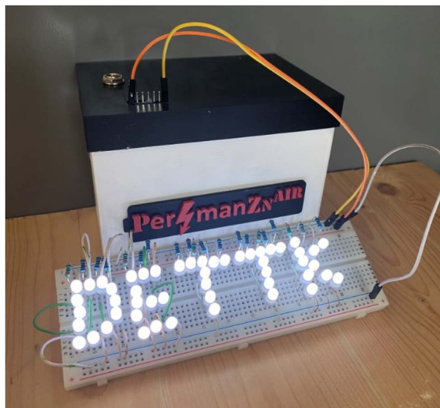
Fig. 5 The prototype battery, with six zinc–O 2 (ads) cells connected in series powering the text 'DE TTK' (the acronym for our university and faculty in Hungarian), formed by 51 LEDs.
