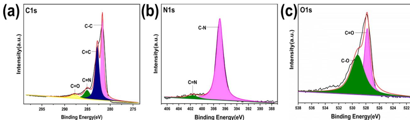
Fig. 7 High-resolution XPS spectra of COF-3: (a) carbon atom, (b) nitrogen atom, and (c) oxygen atom.
