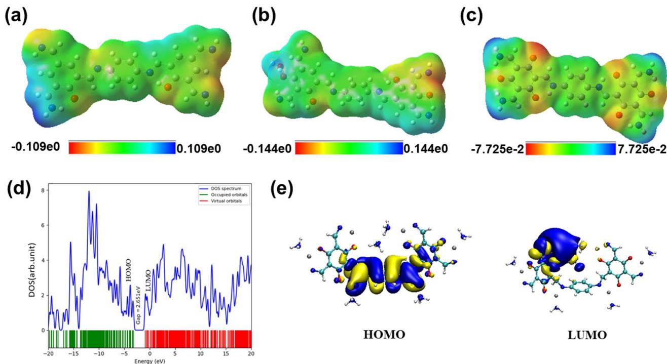
Fig. 13 Adsorption energies for (a) Zn@COF-1@NH<sub>3</sub>, (b) Zn@COF-2@NH<sub>3</sub>, and (c) Zn@COF-3@NH<sub>3</sub>. (d) Density of states for Zn@COF-3, and (e) HOMO–LUMO plots of Zn@COF-3.
