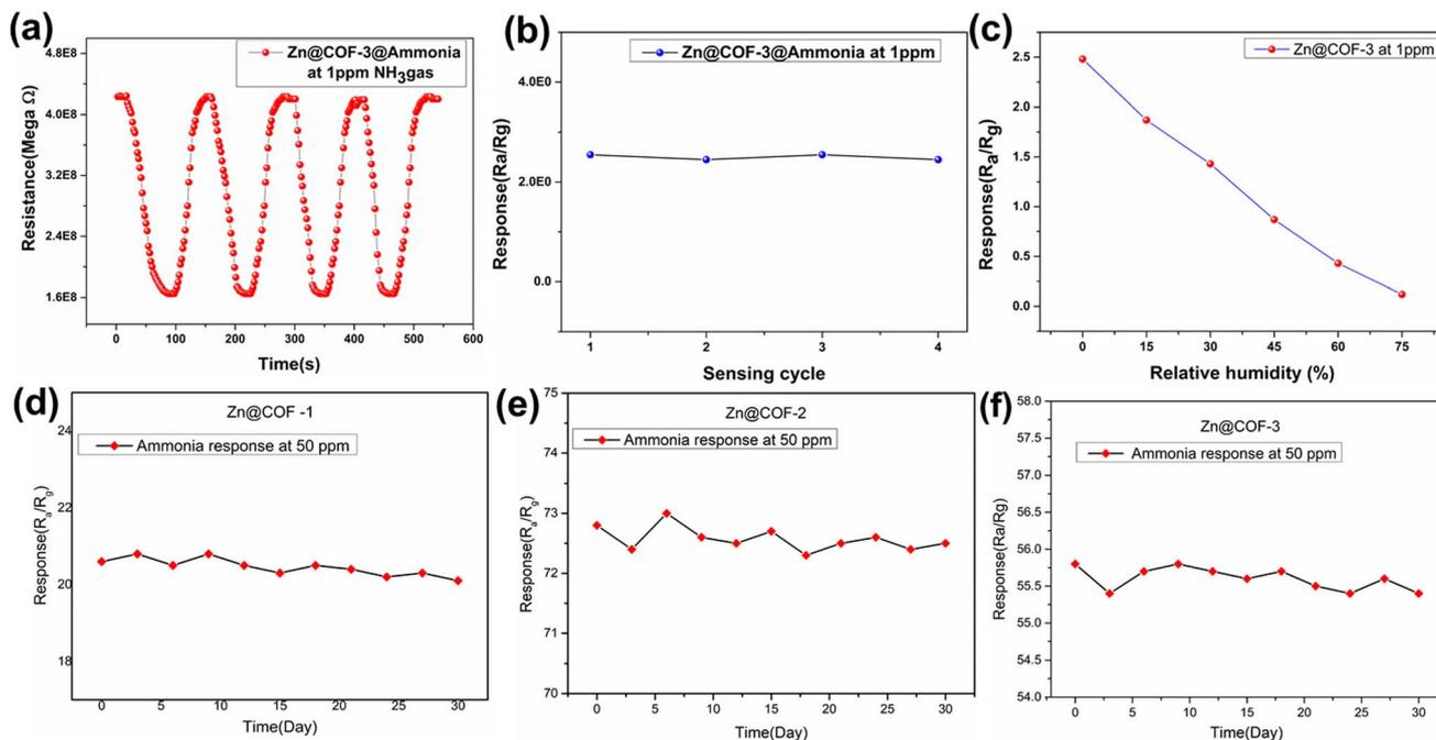
Fig. 11 (a and b) Reproducibility of Zn@COF-3 at 1 ppm. (c) Response ( $R_a/R_g$ ) of the Zn@COF-3 sensor to 1 ppm of ammonia gas under varying relative humidity (RH) conditions. (d–f) Long-term stability of the responses of Zn@COF-1, Zn@COF-2, and Zn@COF-3 towards ammonia gas at 50 ppm.
