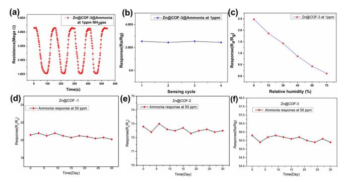
Fig. 11 (a and b) Reproducibility of Zn@COF-3 at 1 ppm. (c) Response  $(R_a/R_a)$  of the Zn@COF-3 sensor to 1 ppm of ammonia gas under varying relative humidity (RH) conditions. (d-f) Long-term stability of the responses of Zn@COF-1, Zn@COF-2, and Zn@COF-3 towards ammonia gas at 50 ppm.
