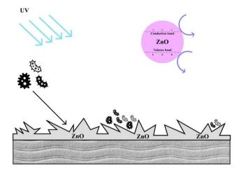
Fig. 22 Soil release finished using ZnO nanoparticle. Published under CC-BY License<sup>168</sup> Copyright 2025, Springer Nature.
