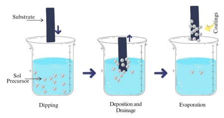
Fig. 2 Dip-coating mechanism.
