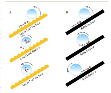
Fig. 18 Diagrammatic representation of the "self-cleaning" idea. A drop of water rolling over the surface of a lotus leaf (A) and a smooth, solid surface (B). Reproduced with permission from ref. 102 Copyright 2022, Springer Nature Switzerland AG.
