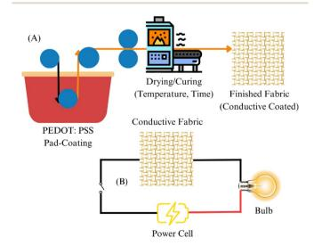
21 Diagrammatic representation of: (A) poly-3,4-ethylenedioxythiphene:polystyrene sulfonate (PEDOD:PSS) continuous coating process; (B) electrical conductivity testing of pretreated fabric. Published under CC-BY License<sup>123</sup> Copy 2022, MDPI.
