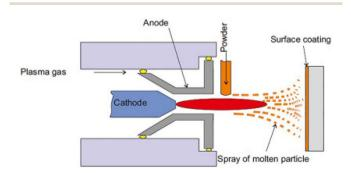
Fig. 4 Plasma treatment mechanism. Reproduced with permission from ref. 31 Copyright 2021, Elsevier Ltd.
