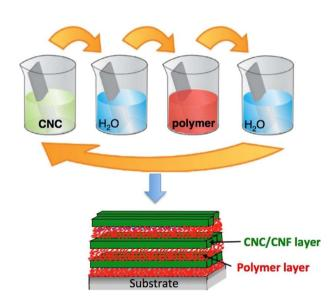
Fig. 6 Layer-by-Layer assembly. Reproduced with permission from ref. 39 Copyright 2018, De Gruyter.
