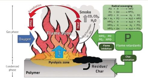
Fig. 8 Flaming combustion of polymeric material and the role of phosphorus-based flame retardants. Published under CC-BY-NC License<sup>45</sup> Copyright 2018, Wiley-VCH Verlag GmbH & Co. KGaA, Weinheim.
