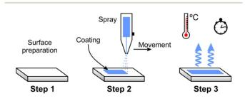
Fig. 3 Spray-coating setup. Reproduced with permission from ref. 28 Copyright 2020, Springer-Verlag GmbH Germany, part of Springer Nature.
