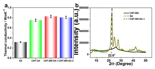
Fig. 3 (a) the thermal conductivity of SA, CNT-SA, CNT-BN-SA-1, and CNT-BN-SA-2 (b) the XRD diffractogram of CNT-BN, SA and CNT-BN-SA-1.
