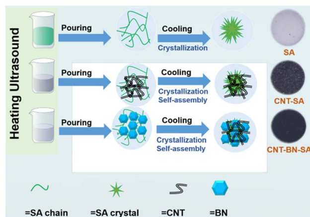
Fig. 1 Preparation process of SA, CNT-SA, and CNT-BN-SA.
