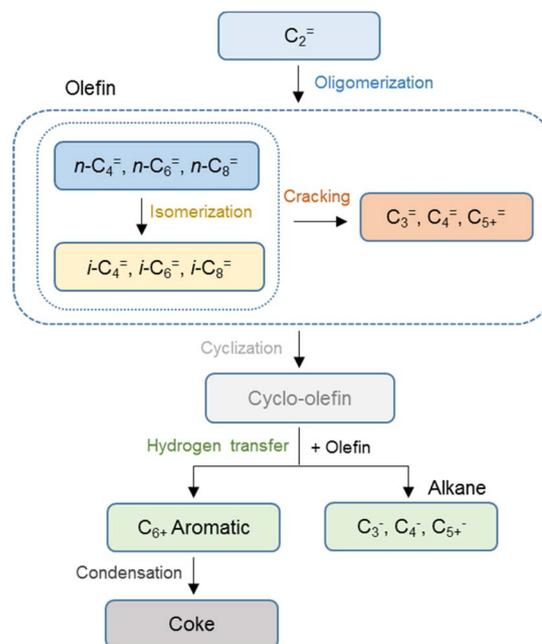
Scheme 1 Simplified reaction pathways for ethylene oligomerization over zeolite catalysts.
