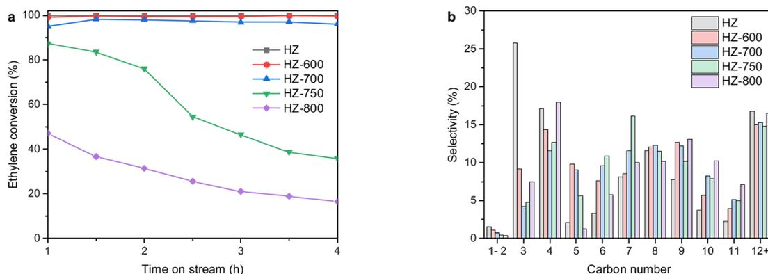
Fig. 6 (a) Evolution of ethylene conversion and (b) product distribution of carbon number with time on stream of 4 h over steam modified ZSM-5 samples.
