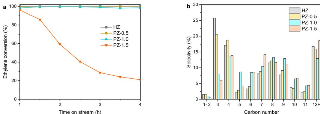
Fig. 7 (a) Evolution of ethylene conversion and (b) product distribution of carbon number with time on stream of 4 h over phosphorus modified ZSM-5 samples.
