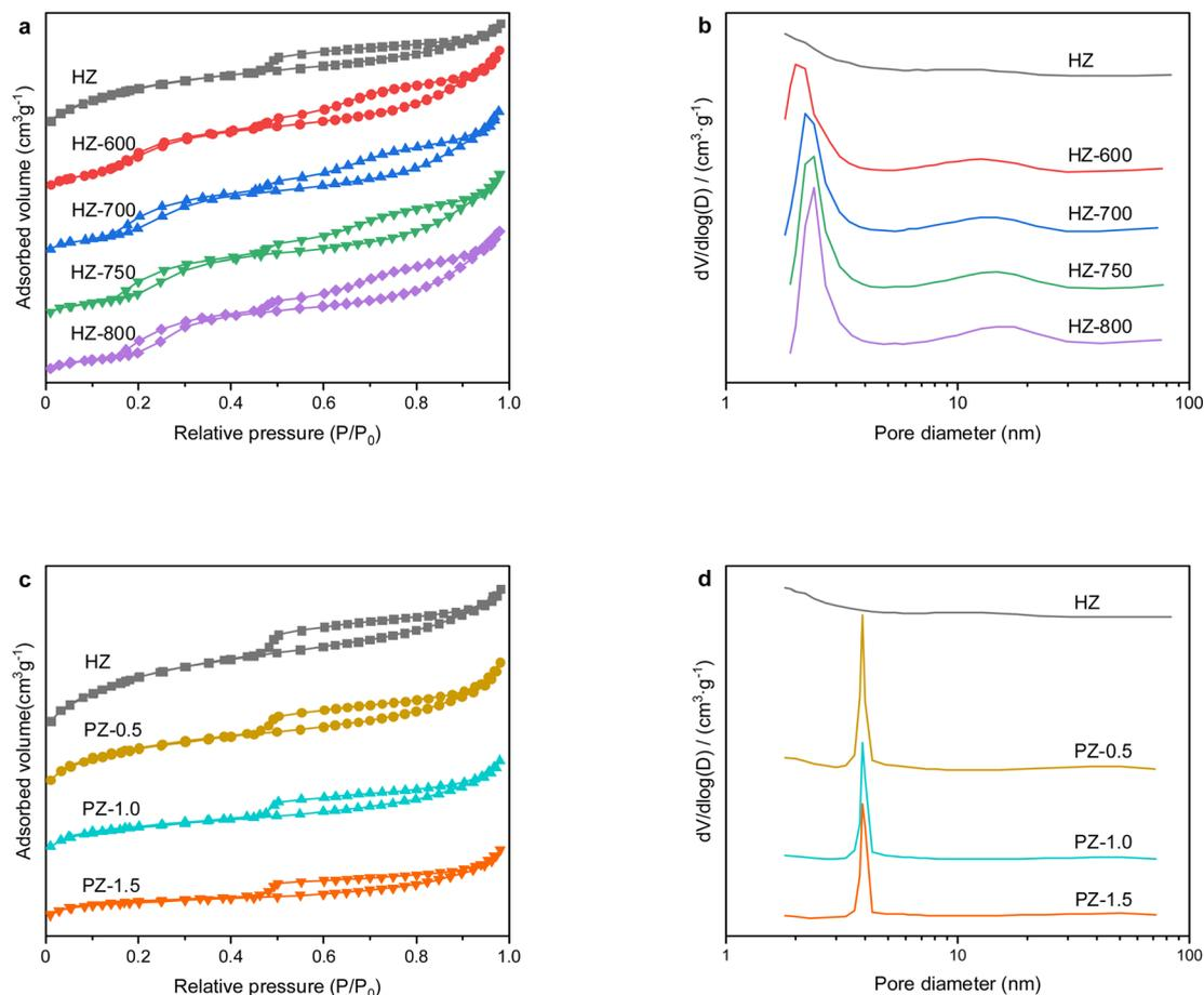
Fig. 2 N<sub>2</sub> adsorption–desorption isotherms and pore size distribution of (a and b) steam and (c and d) phosphorus modified ZSM-5 samples.
