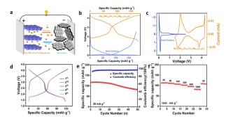
Fig. 4 Sodium-ion full batteries: (a) schematic configuration of the P2-NFMO-CoMgLi cathode//hard carbon anode full battery. (b) Charge/discharge pro-files and (c) CV curves of the P2-NFMO-CoMgLi cathode and hard carbon anode. (d) Galvanostatic charge/discharge profiles and (e) cycling performance at 0.1C in the voltage window of 1.4–4.1 V of the full cell (based on the cathode active mass). (f) Rate performance of the full battery.
