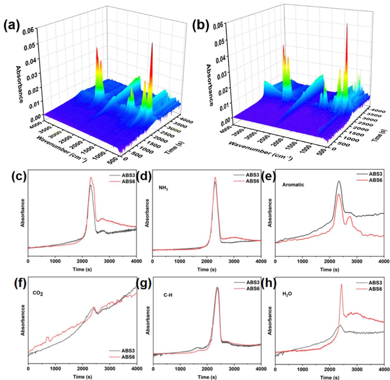
Fig. 9 3D Fourier infrared spectrum spectra of ABS3 (a) and ABS6 (b). FTIR spectra of the total gaseous products (c). Absorption intensities of pyrolysis gases of ABS3 and ABS6 (d–h).
