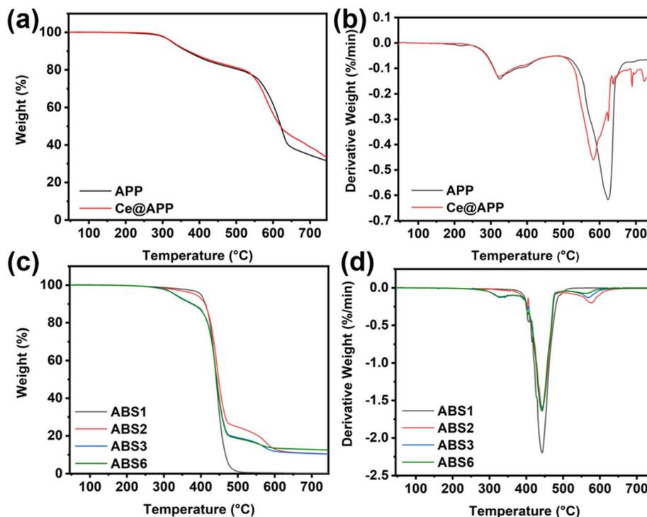
Fig. 4 TG (a) and DTG (b) curves of APP and Ce@APP. TG (c) and DTG (d) curves of ABS composites.
