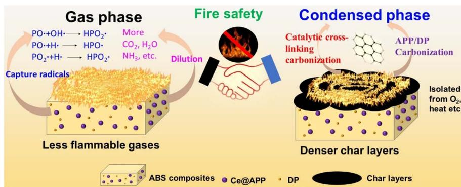
Fig. 10 Possible flame-retardant mechanism of Ce@APP/DP in ABS.
