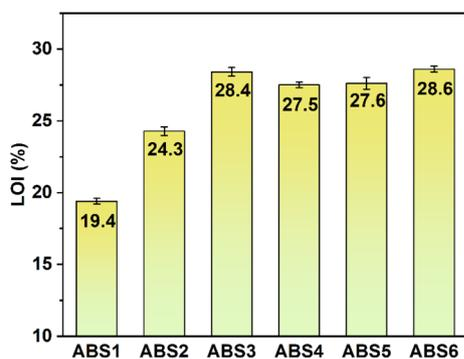
Fig. 5 LOI and UL-94 curves of ABS composites.
