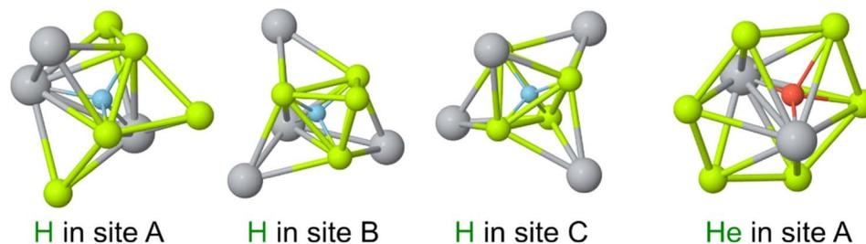
Fig. 1 Stable interstitial hydrogen and helium sites within the crystal lattice of  $\text{Be}_2\text{Ti}$ . Only beryllium and titanium atoms located within a 2.90 Å radius from the interstitial are displayed. Interstitial hydrogen and helium atoms are connected to the nearest beryllium and titanium atoms by thin lines to indicate their precise positions in the lattice.
