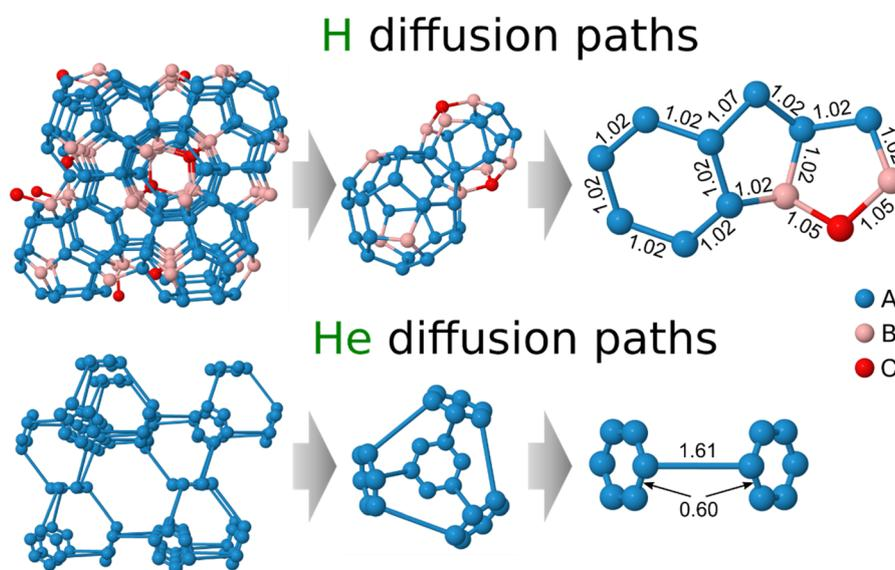
Fig. 2 The stable interstitial hydrogen (top) and helium (bottom) sites within the crystal lattice of  $\text{Be}_2\text{Ti}$ . The main diffusion path patterns formed by regular polygons, along with all non-equivalent polygons forming polyhedra, are presented. Bonds between neighboring stable interstitial sites illustrate possible diffusion jumps (in Å).
