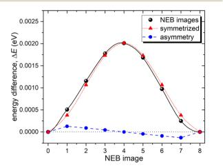
Fig. 4 The energy barrier between adjacent non-equivalent interstitial helium sites A for intra-hexagonal jump calculated using NEB method. For comparison, a symmetrized jump and the corresponding asymmetry are also presented. Horizontal dotted line and the solid lines connecting the data points serve as a guide to the eye.
