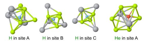
Fig. 1 Stable interstitial hydrogen and helium sites within the crystal lattice of Be<sub>2</sub>Ti. Only beryllium and titanium atoms located within a 2.90 Å radius from the interstitial are displayed. Interstitial hydrogen and helium atoms are connected to the nearest beryllium and titanium atoms by thin lines to indicate their precise positions in the lattice.
