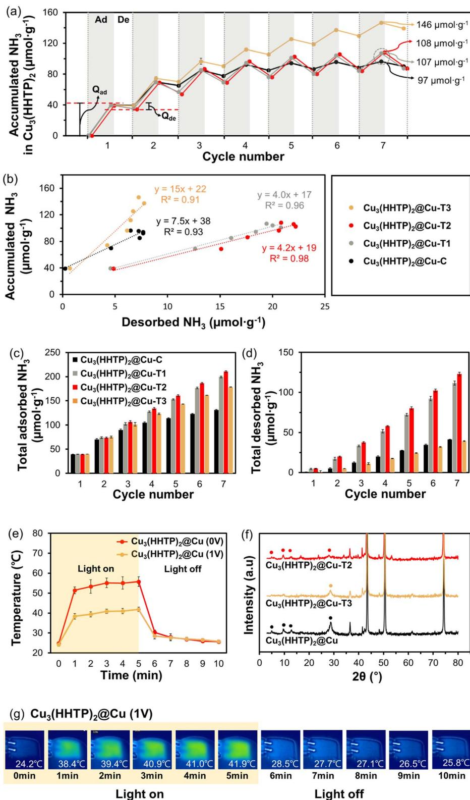
Fig. 8 (a) Cyclic process of  $\text{NH}_3$  adsorption–desorption, (b) accumulated  $\text{NH}_3$  retained under different treatment conditions, (c) total  $\text{NH}_3$  adsorption per cycle (without desorption), (d) total  $\text{NH}_3$  desorbed per cycle, (e) photothermal effect with and without 1 V, (f) X-ray diffraction (XRD) patterns of  $\text{Cu}_3(\text{HHTP})_2@Cu$ . (g) Infrared images after 1 V application.
