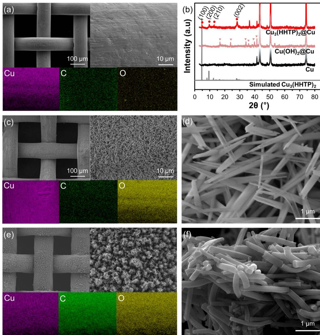
Fig. 1 Scanning electron microscopy (SEM) images and elemental mapping of (a) Cu mesh, (c and d) Cu(OH)<sub>2</sub>@Cu, (e and f) Cu<sub>3</sub>(HHTP)<sub>2</sub>@Cu, and (b) X-ray diffraction (XRD) patterns.
