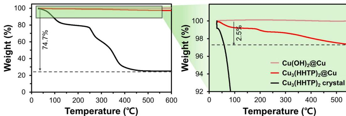
Fig. 2 Thermogravimetric analysis (TGA) curve of Cu<sub>3</sub>(HHTP)<sub>2</sub>.
