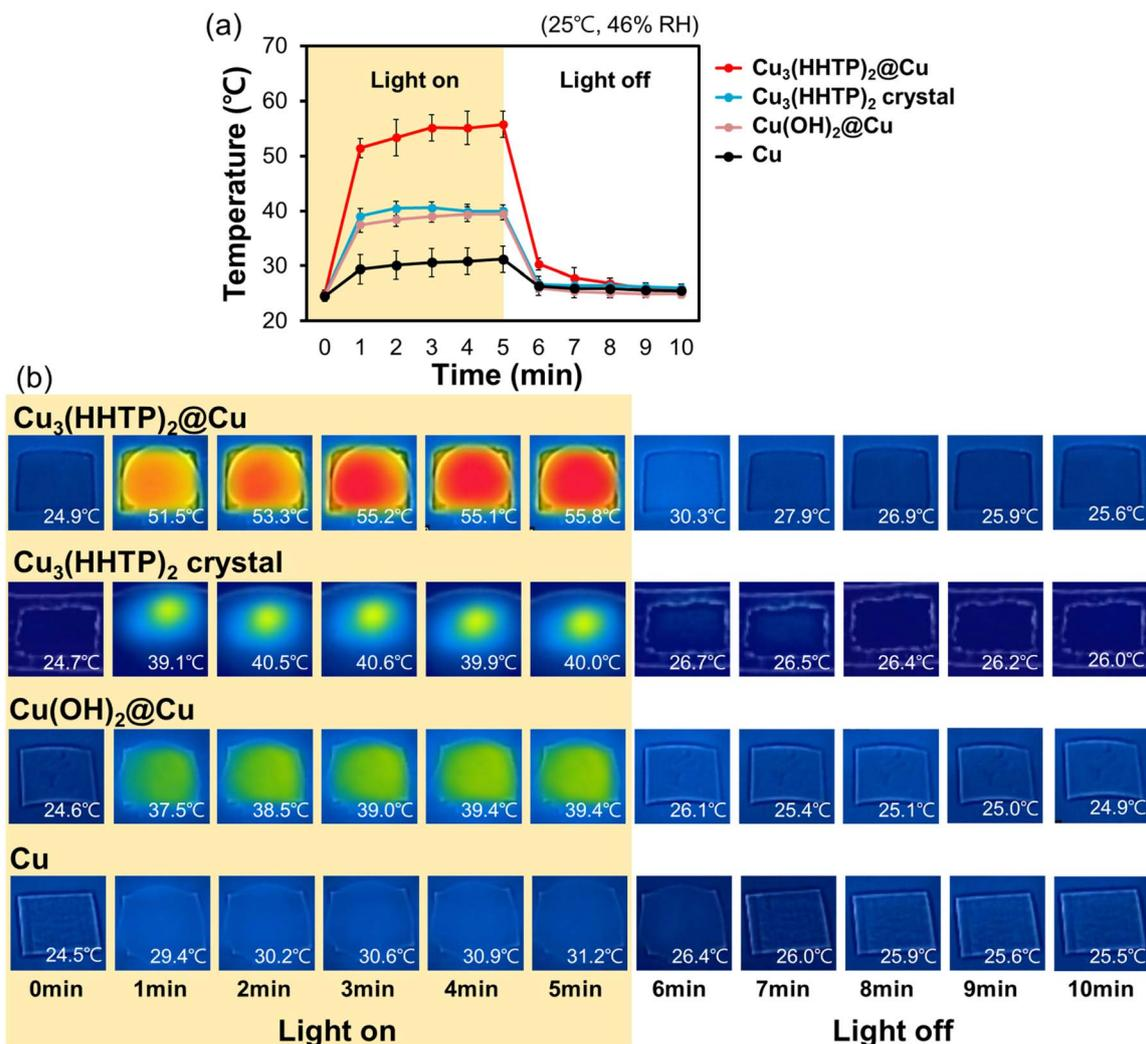
**Fig. 7** Photothermal conversion effects demonstrated by (a) surface temperature changes and (b) infrared images for Cu, Cu(OH)<sub>2</sub>@Cu, Cu<sub>3</sub>(HHTP)<sub>2</sub> crystal, and Cu<sub>3</sub>(HHTP)<sub>2</sub>@Cu.
