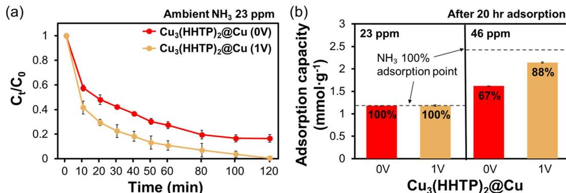
Fig. 3  $\text{NH}_3$  adsorption with and without voltage. (a)  $\text{NH}_3$  adsorption for 2 h at 23 ppm  $\text{NH}_3$ , (b)  $\text{NH}_3$  adsorption efficiency (%) and capacity per g of  $\text{Cu}_3(\text{HHTP})_2$  crystals attached on Cu mesh under 23 ppm and 46 ppm  $\text{NH}_3$ .
