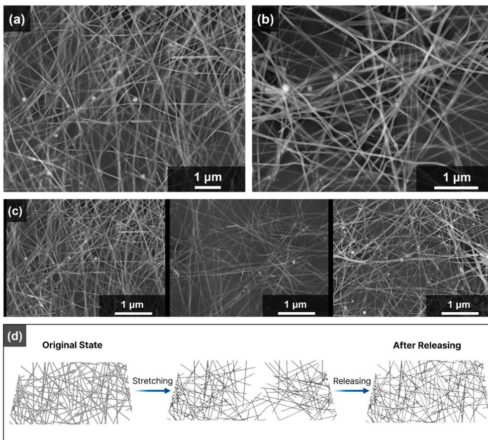
Fig. 5 FE-SEM images of the simple-structured PIS/AgNW composite film surfaces at (a) 150 00 $\times$  and (b) 250 00 $\times$  magnification. (c) FE-SEM images of surface morphology for the simple-structured films before stretching (left), under a strain of ca. 10% (middle), and after releasing (right). (d) Illustration of AgNW conductive paths upon stretching/releasing.
