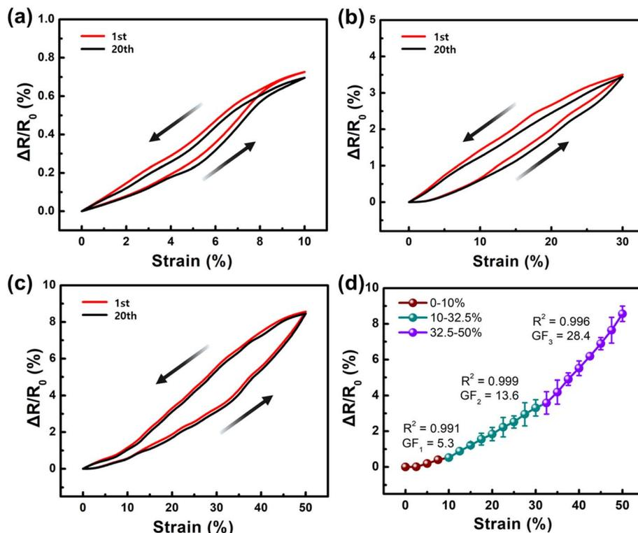
Fig. 6 Relative resistance variations ( $\Delta R/R_0$ ) of the sandwich-structured PIS/AgNW/PIS composite films under (a) 10%, (b) 30%, and (c) 50% strain during the first and the 20th stretching/releasing cycles. (d) The  $\Delta R/R_0$  of the sandwich-structured films versus the applied strain up to 50% and the corresponding gauge factors.
