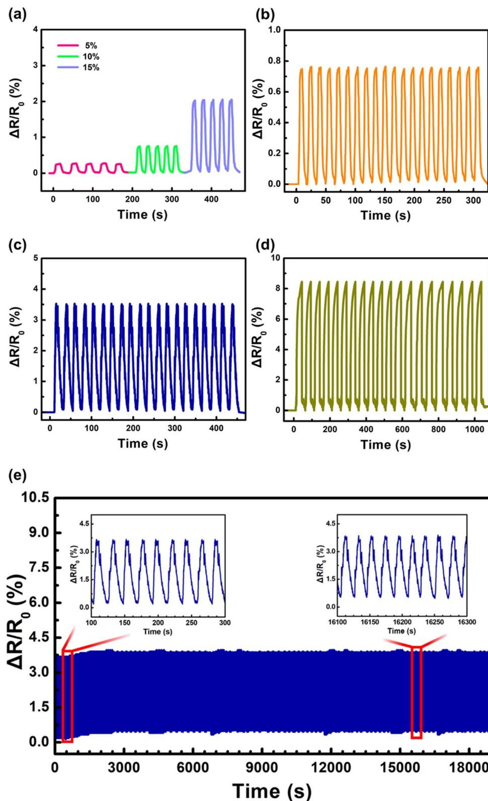
Fig. 7 (a) Relative resistance variation ( $\Delta R/R_0$ ) of the sandwich-structured PIS/AgNW/PIS composite films versus time with a stepwise increase in strain from 5% to 15%. Response of the sandwich-structured films under (b) 10%, (c) 30%, (d) 50% strain during 20 stretching/releasing cycles, and (e) 30% strain during 1000 stretching/releasing cycles.
