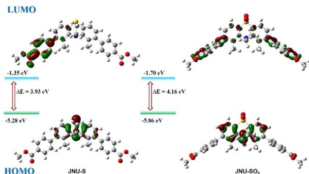
Fig. 5 Optimized structures of JNU-S (left) and JNU-SO<sub>2</sub> (right), their HOMO–LUMO and orbital energies were calculated using the B3LYP/6-31G(d,p) basis set.
