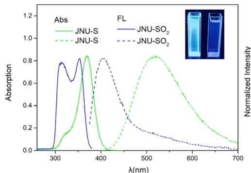
Fig. 6 Normalized absorption (solid) and emission (dash) spectra of JNU-S ( $\lambda_{\text{ex}} = 370$  nm) and JNU-SO<sub>2</sub> ( $\lambda_{\text{ex}} = 355$  nm) in CHCl<sub>3</sub> ( $c = 2.0 \times 10^{-3}$  mol L<sup>-1</sup>).
