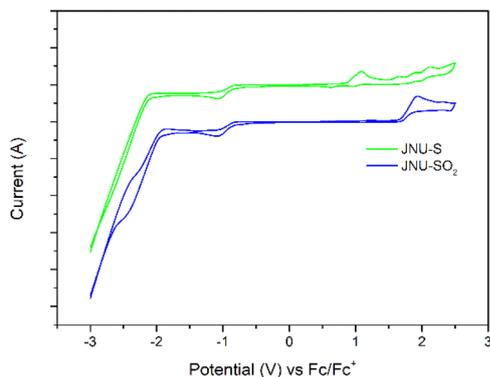
Fig. 4 Cyclic voltammograms of JNU (green) and JNU-SO<sub>2</sub> (blue) in 0.1 M solution of Bu<sub>4</sub>NPF<sub>6</sub> in dichloromethane at 50 mV s<sup>-1</sup> scan rate versus vs. Ag/AgCl at 25 °C.
